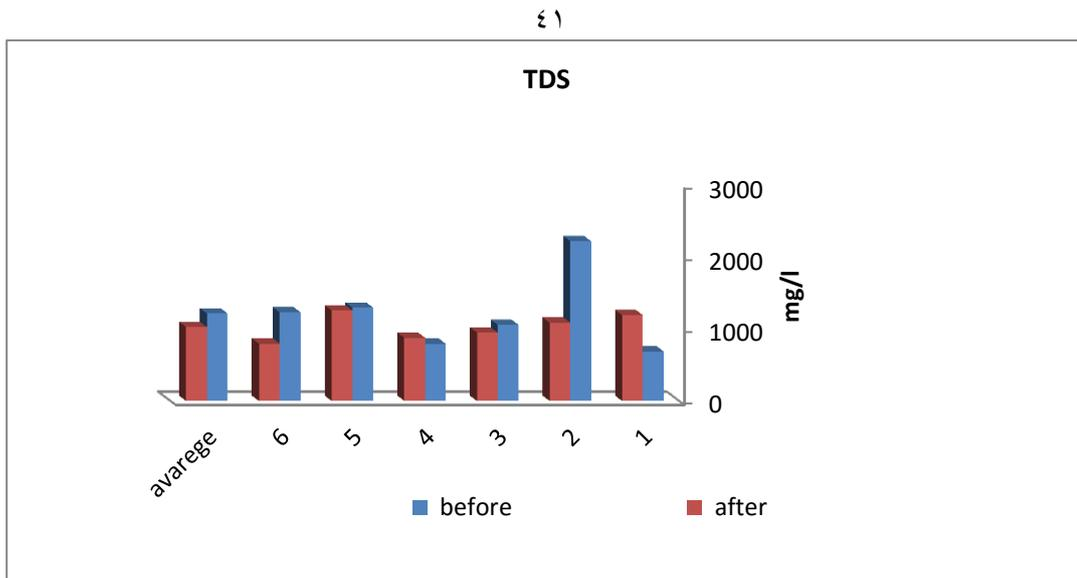
**Figure(٤.٨):** Values of Measured TDS before and after treatment from the six targeted treatment plants.
