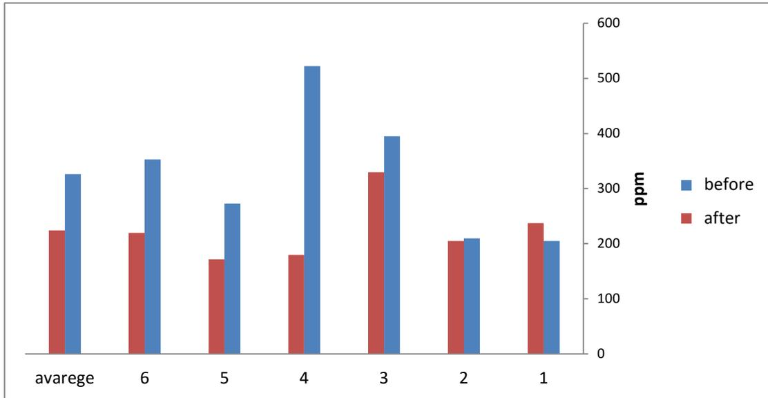
**Figure (٤.٦):** Values of Measured  $Cl^-$  before and after treatment from the six targeted treatment plants.
