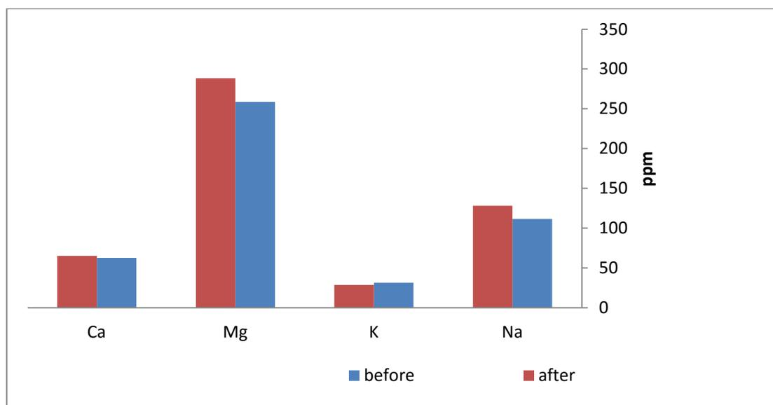
**Figure(٤.١٢):** Overall average values of  $Mg^{2+}$ ,  $Ca^{2+}$ ,  $K^+$  and  $Na^+$  measured for treated greywater.
