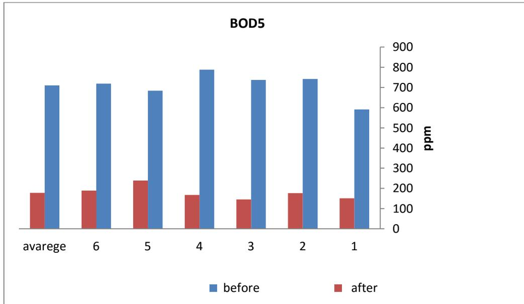
**Figure (٤.٢):** Values of Measured BOD<sup>o</sup> before and after treatment water from the six targeted treatment plants.
