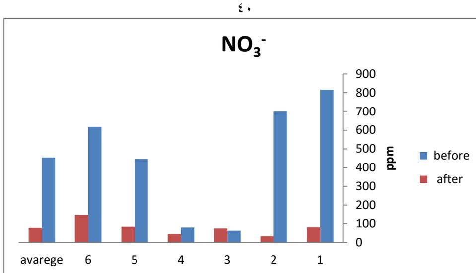
**Figure(٤.٧):** Values of Measured NO<sub>3</sub><sup>-</sup> before and after treatment from the six targeted treatment plants.
