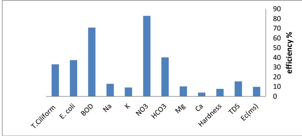
**Figure (٤. ١٣):** Efficiency of Treated Greywater System as Percent Removal
