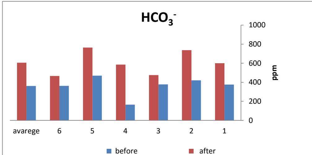
**Figure (٣. ٥):** Values of Measured HCO<sub>3</sub><sup>-</sup> before and after treatment from the six targeted treatment plants.
