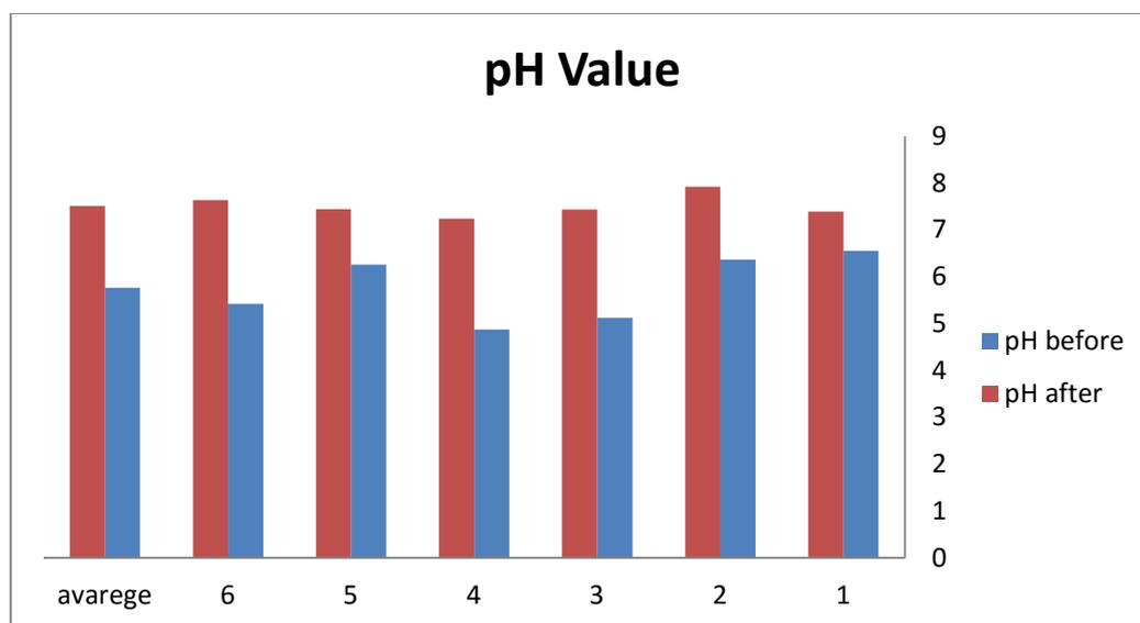
**Figure(٤.٩):**Values of Measured pH before and after treatment from the six targeted treatment plants.
