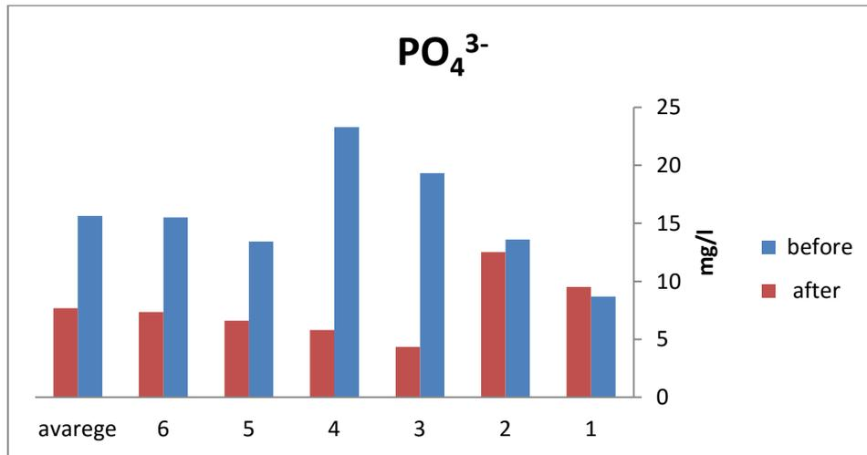
**Figure (٤. ٣):** Values of Measured PO<sub>4</sub><sup>3-</sup> before and after treatment from the six targeted treatment plants.
