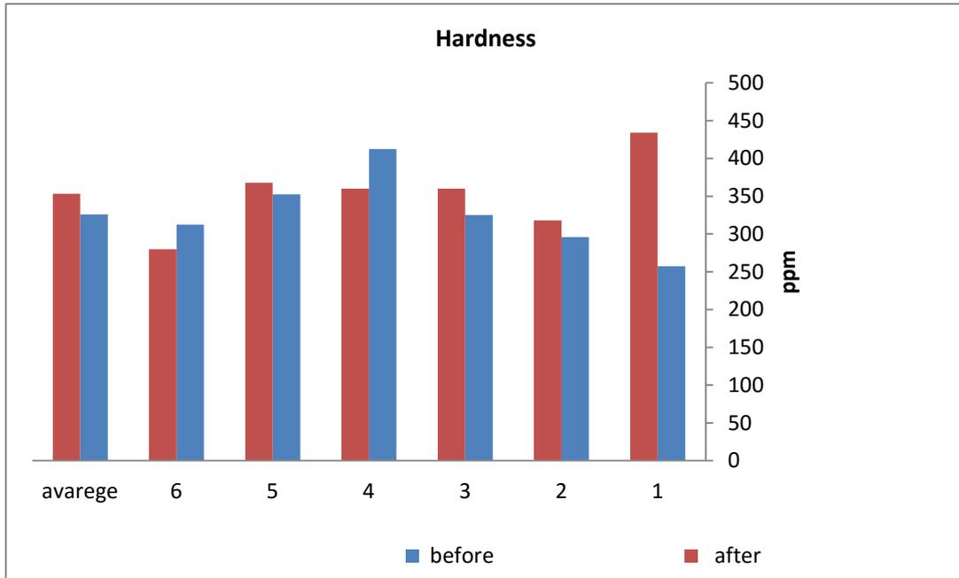
**Figure (٤.٤):** Values of Measured Hardness before and after treatment from the six targeted treatment plants.
