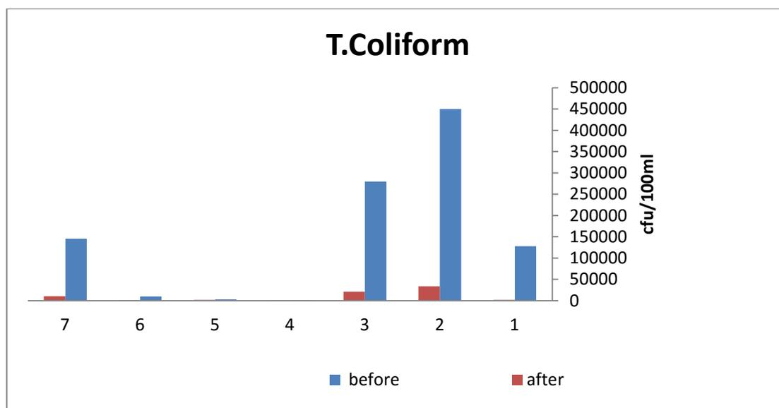
**Figure(٤. ١١):**Values of Measured Total Coliform before and after treatment from the six targeted treatment plants.
