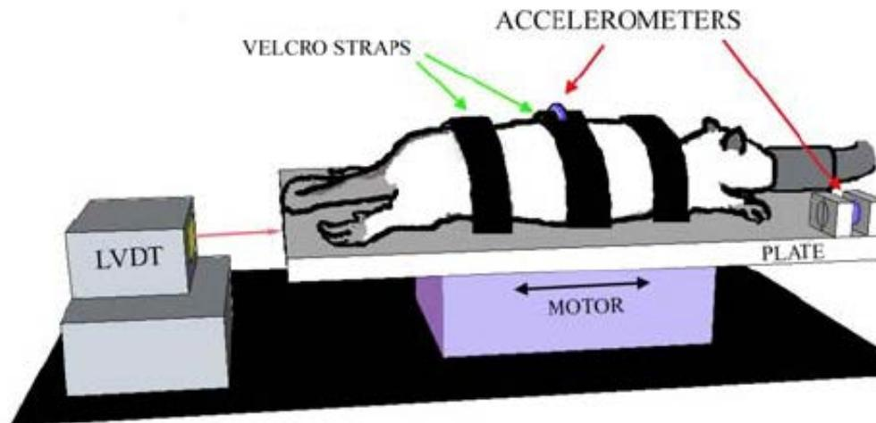
Fig. 2. Schematic of WBV device, indicating the set-up and instrumentation.
