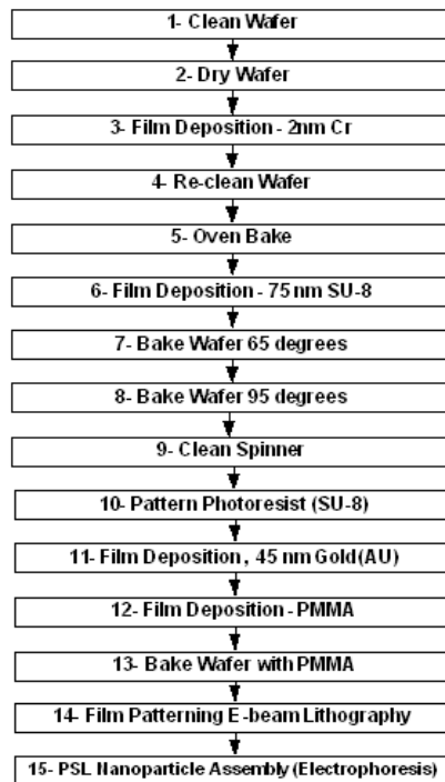
Figure 3: Fifteen process steps for fabrication of a PSL biosensor
