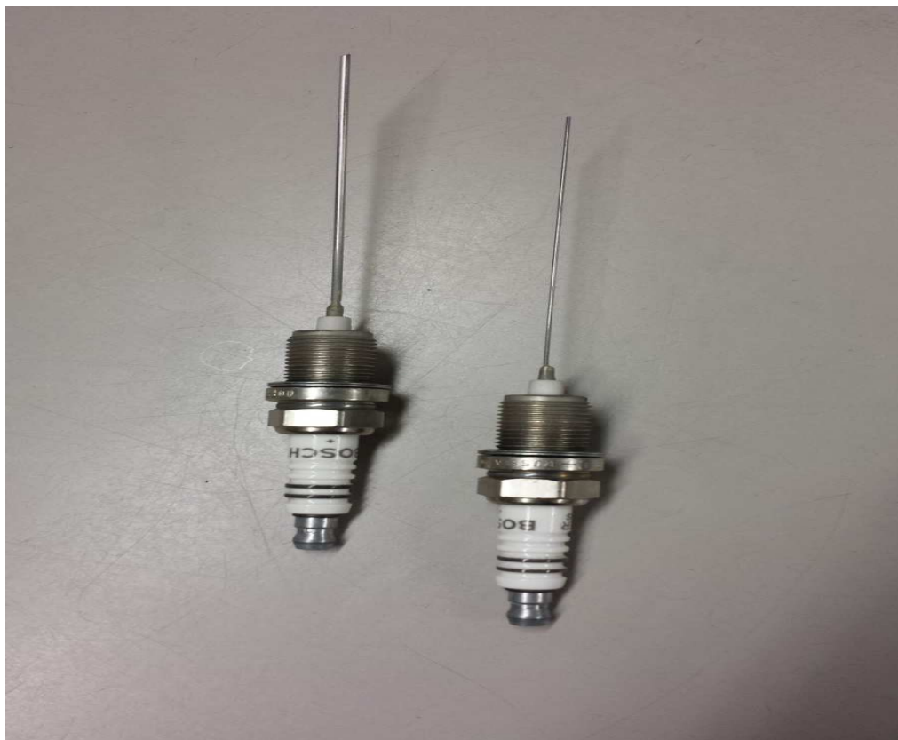
Figure 4: Typical automotive spark plugs modified with extended electrode for use in combustion vessels.
