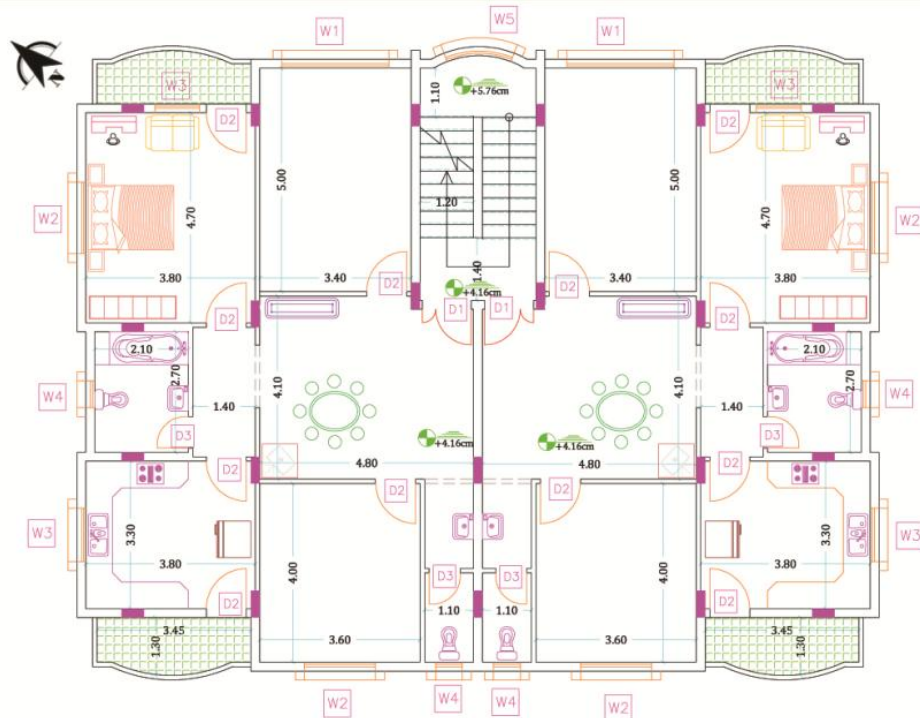
Figure (3.29): Plan of 2 floor separate house with 2 apartment in each floor Source: Al-Rabwa Engineering Consultant- Khan Younis, (2012)
