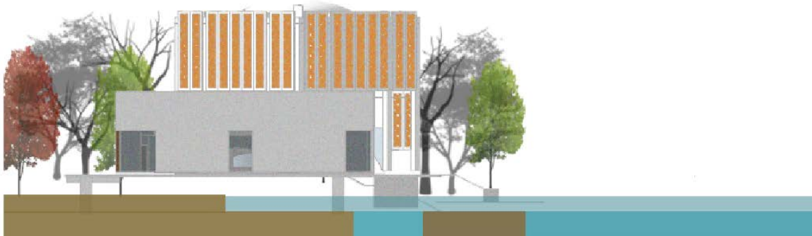
Figure 32- Darker blue representing general water level,lighter blue shows the water level while flooding
