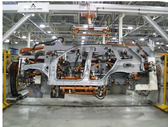
Fig. 2.4. Measurement of side panels of BMW X5 car [10]
