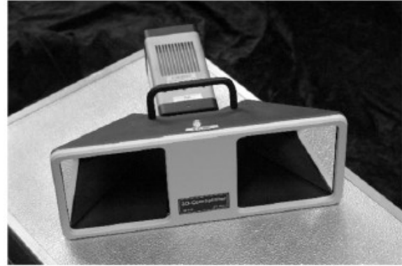
Fig. 5. High-speed camera with stereo beam splitter.
