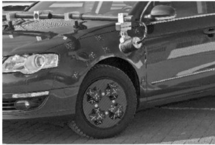
Fig. 4. High-speed camera with FPGA-based target detection (AICON).
