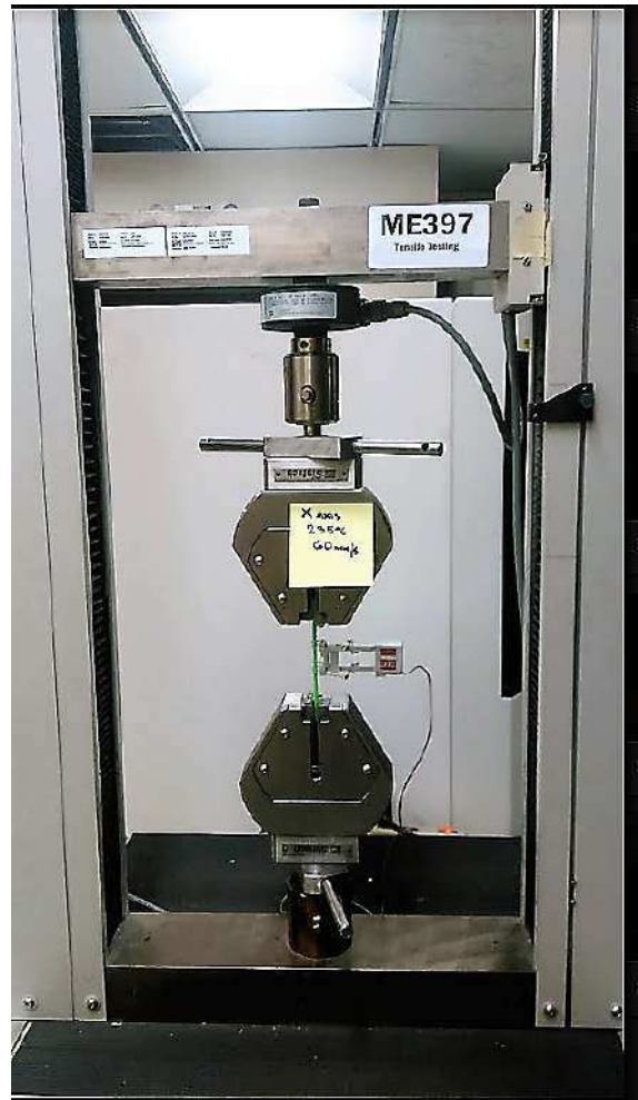
Figure 3.10. Installation of specimen into Q-test machine and extensometer attached to the specimen for mechanical testing.
