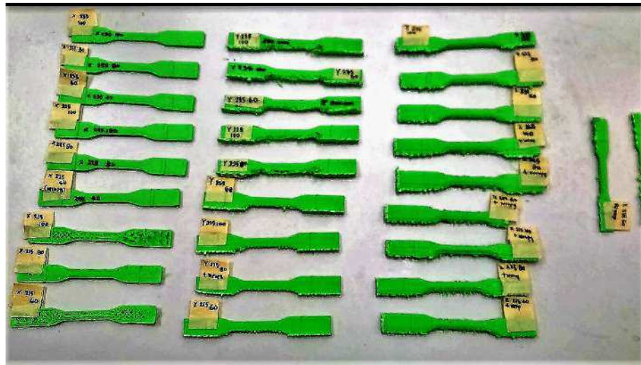
Figure 4.25. Specimen B1 to B27 printed on the AirWolf 3-D printer prior to evaluation on the Q-test machine.
