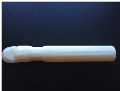
Fig. 2.26. 3D Printed Model of Compression Load Cell Device
