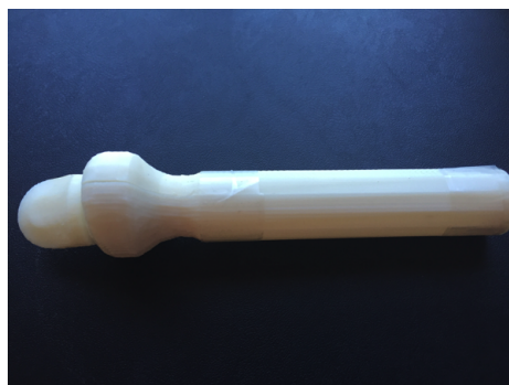
Fig. 2.27. 3D Printed Model of 3D Load Cell Device
