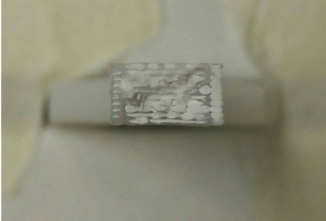
Fig. 2.15. Optical Image of Cross-Section Area of the 0^\circ Tensile Bar Fracture Surface
