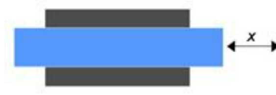
Fig. 2.9. Prismatic joint in 2D
