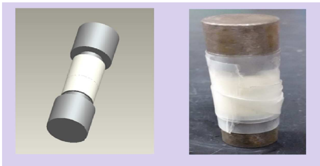
Figure 4.17 Schematic and picture of the device used for testing the cell under pressure
