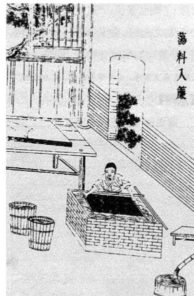
Figure 27 Traditional way of pulling paper from the pulp
