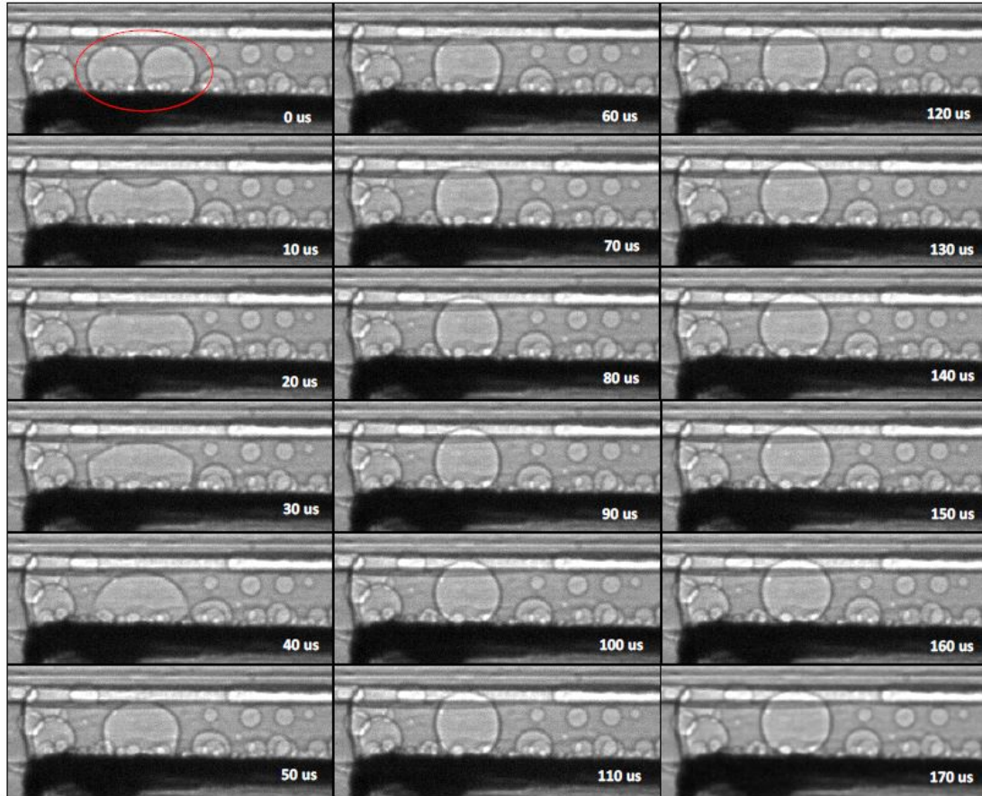
Fig. 2.14. Representative image sequence of equal-sized bubble coalescence. This is case No. 6 mentioned in Table 3.1.
