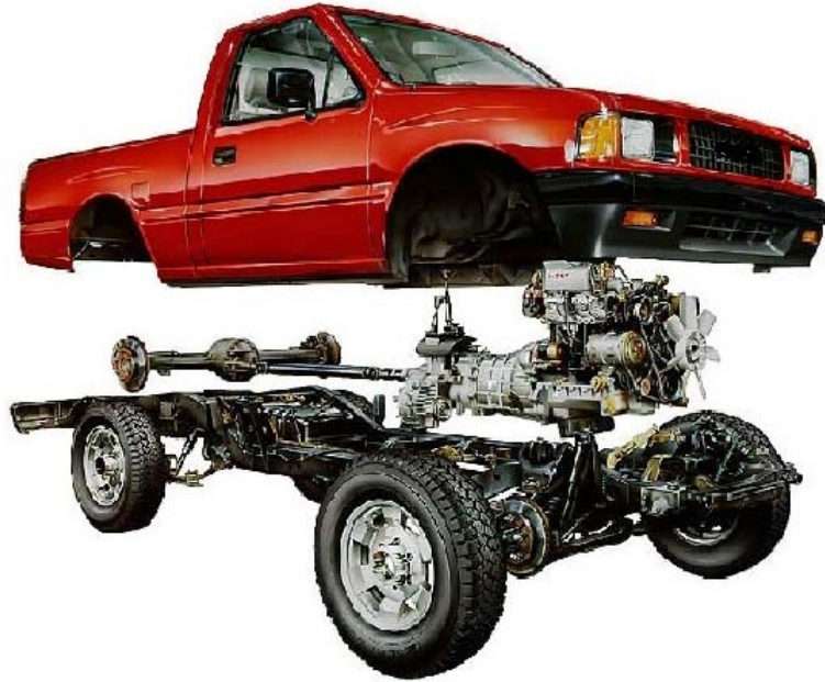
Figure 1.4.: Body-Over-Frame Structure [2]
