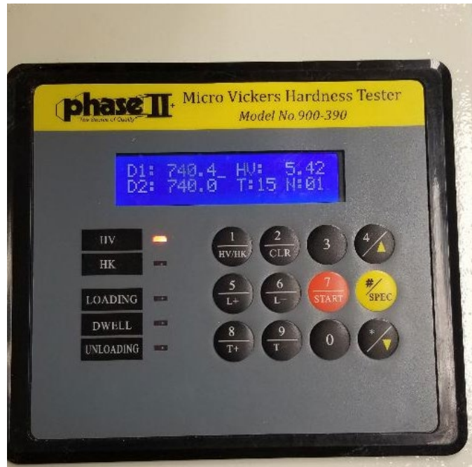
Figure 3.11 Micro Vickers Hardness Tester with data after Indentation with F = 0.98\text{N}
