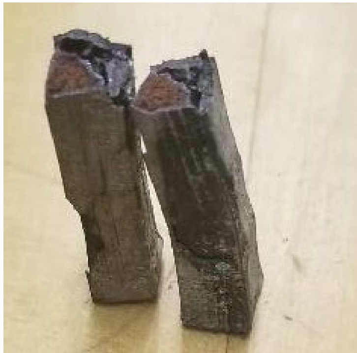
Figure 2.18 Broken Sintered Square Beam
