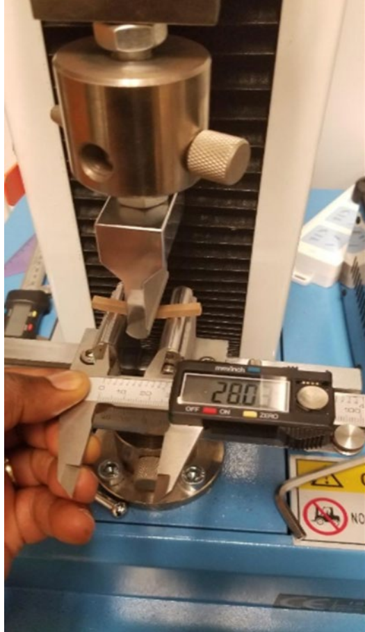
Figure 2.13 3D Printed Square Beam with 28mm Span
