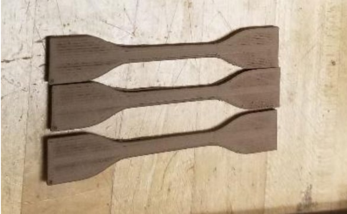
Figure 2.5 Tensile Bar printed with 20% infill density of Bronze Filament
