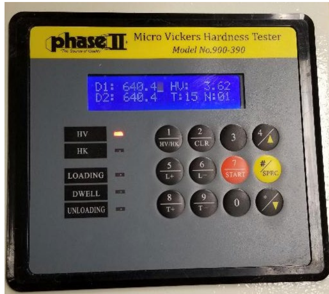
Figure 3.13 Micro Vickers Hardness Tester with data after Indentation with F = 0.49\text{N}
