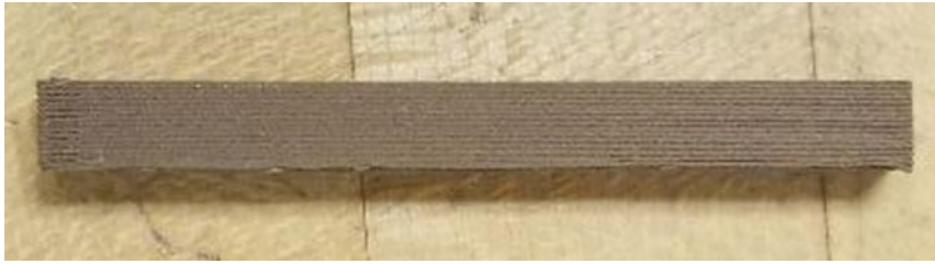
Figure 2.15 Square Beam Printed with 100% infill density of Bronze Filament
