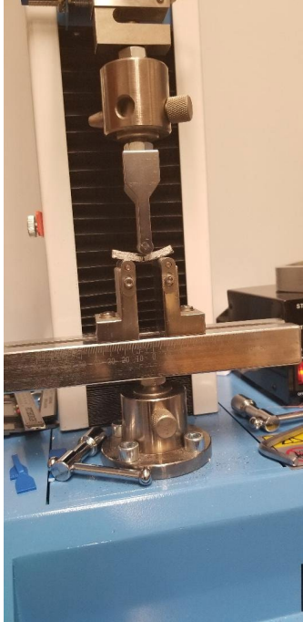
Figure 2.17 Sintered Bronze Square Beam After 3-Point Bending Test
