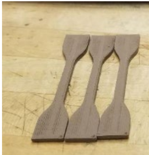
Figure 2.4 Tensile Bar printed with 50% infill density of Bronze Filament
