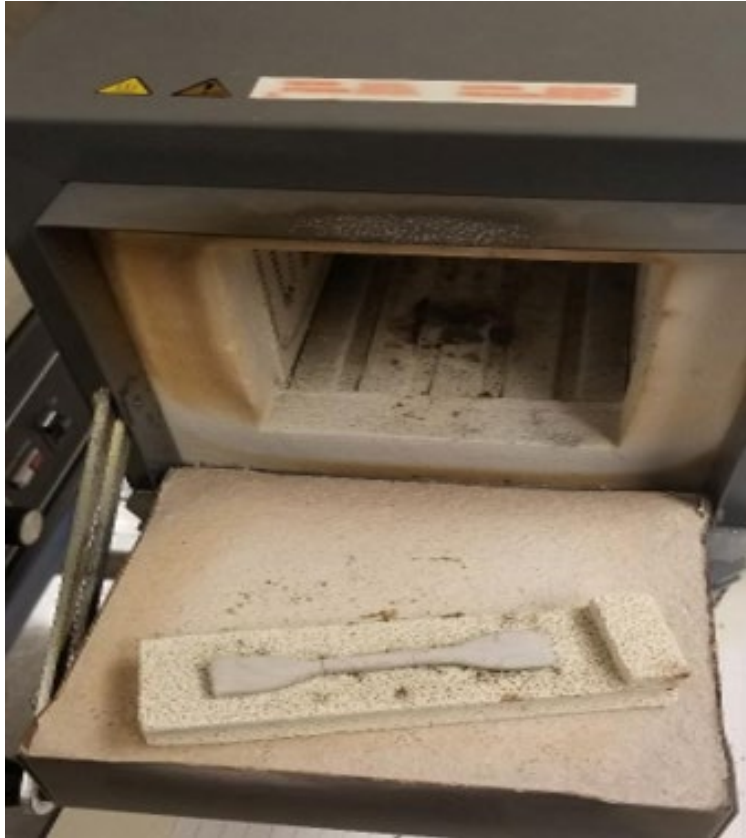
Figure 2.23 Sintered Specimen in the Furnace.
