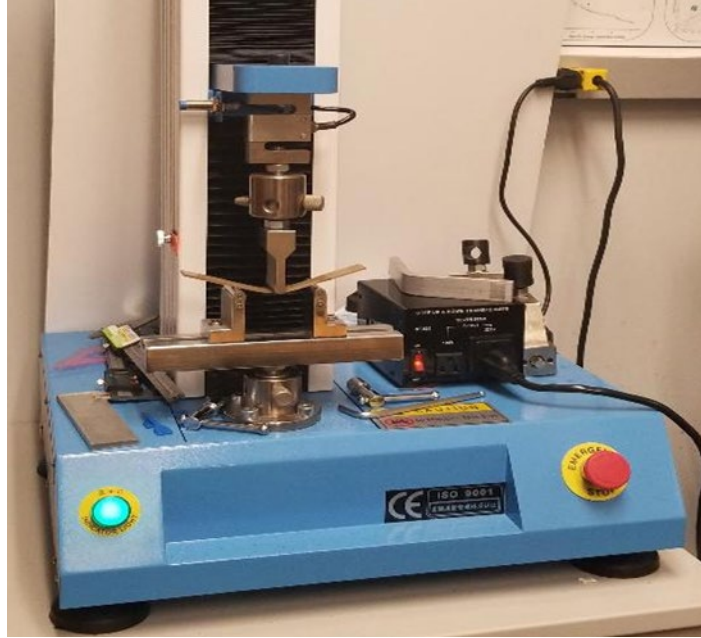
Figure 2.12 Bronze Square Beam After 3-Point Bending Test
