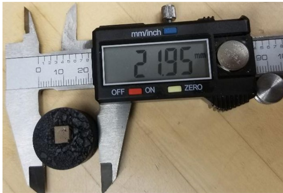
Figure 2.20 3D Printed Bronze specimen placed in black holder for Hardness Test
