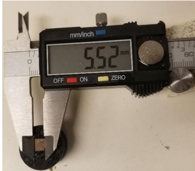
Figure 2.21 3D Printed Bronze specimen prepared for Hardness Test
