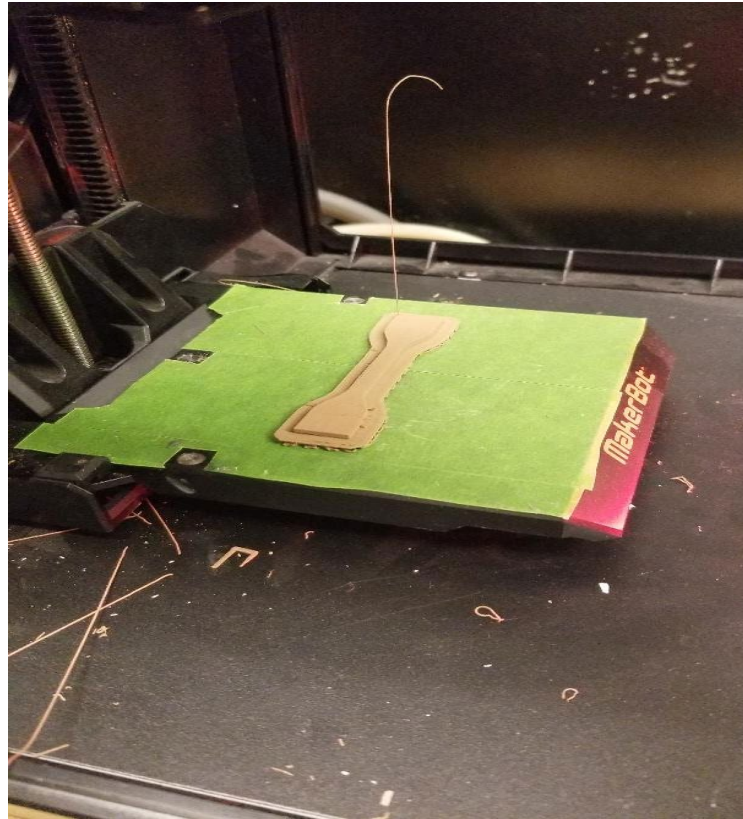
Figure 2.6 Bronze Tensile Bar with the Printed Support.
