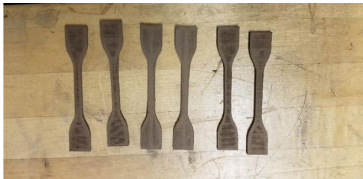
Figure 2.3 Tensile Bar printed with 100% infill density of Bronze Filament
