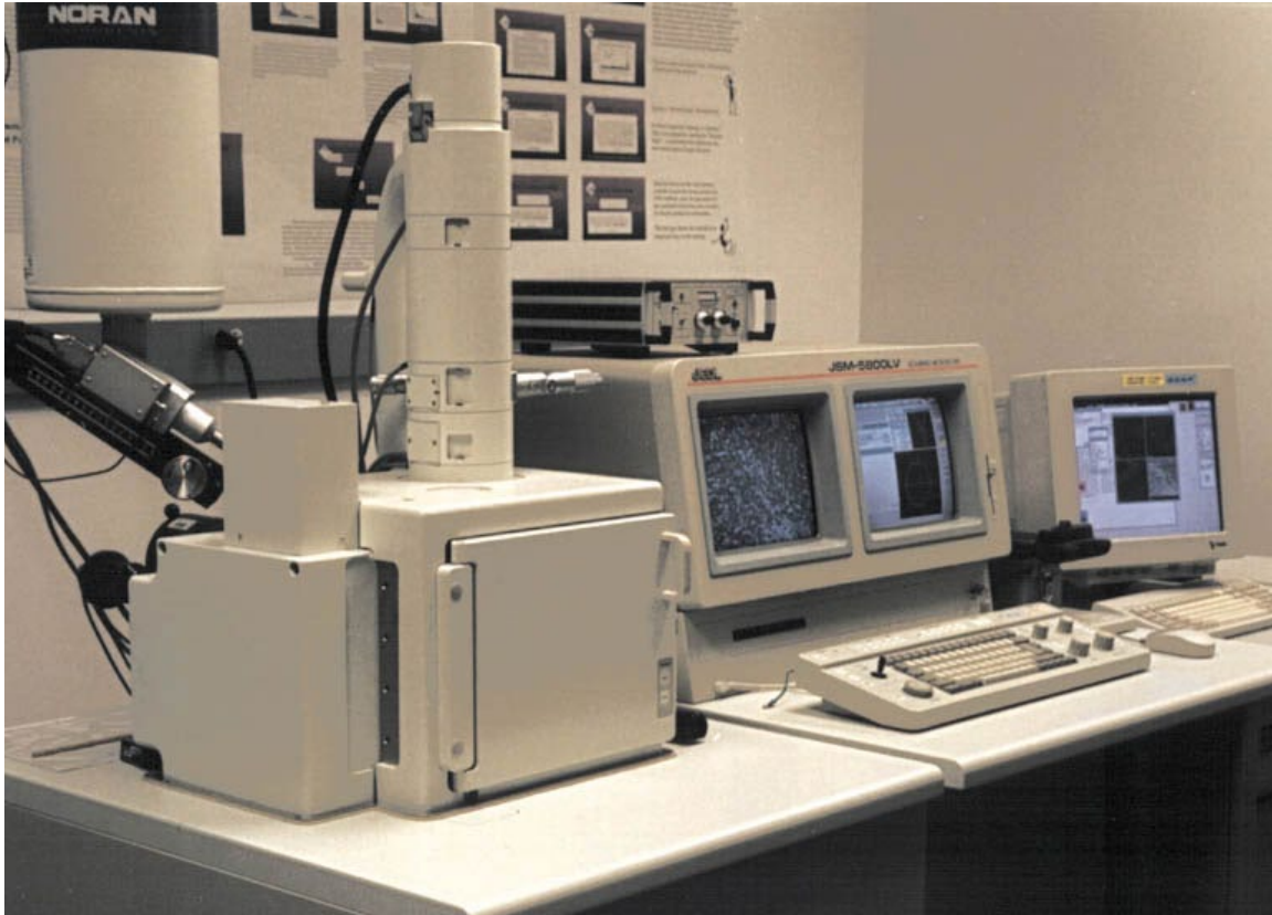
Figure 2.8 Scanning Electron Microscopy (SEM) Instrument [17].
