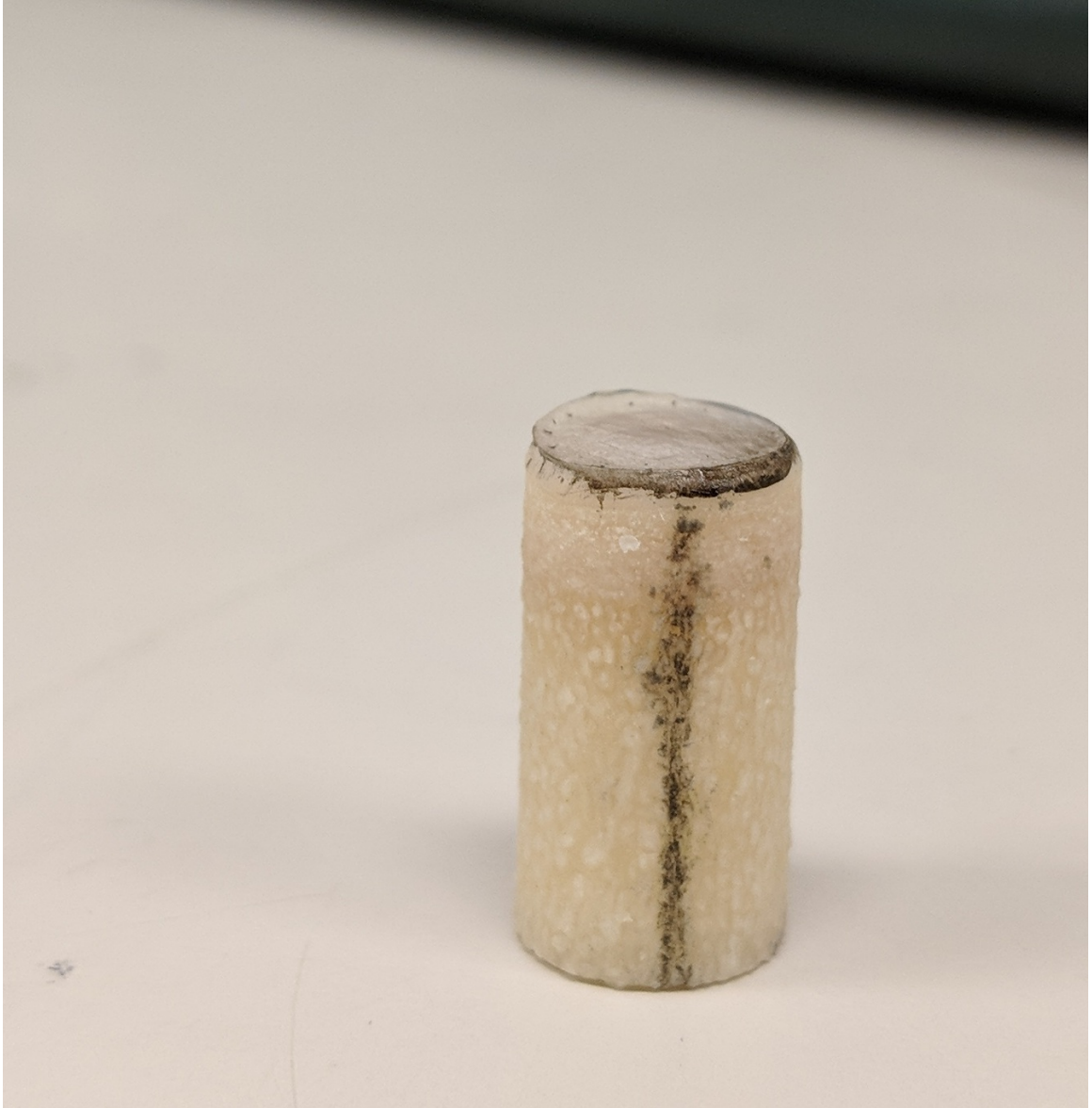
Fig. 2.3. Specimen after complete processing and with marking of fiber direction.
