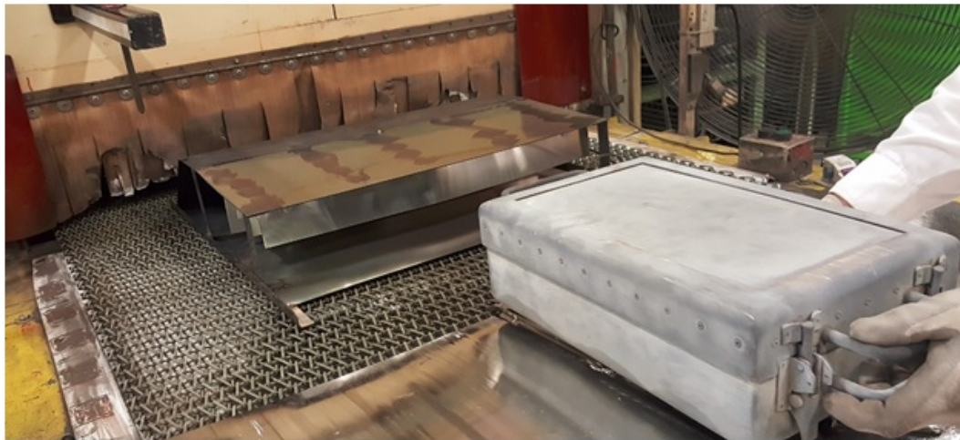
Fig. 3.5. Sample test apparatus with data logger loaded at the start of the furnace.
