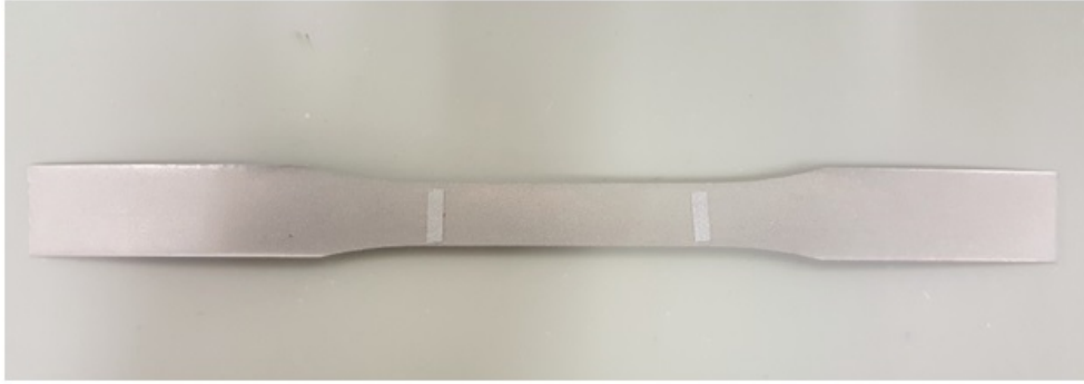
Fig. 3.12. Retro-reflective film (2 inches wide) installed on to every specimen.
