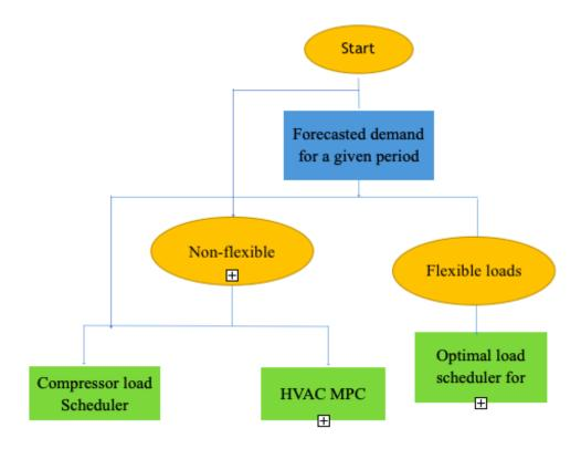
Figure 4.1. Proposed energy management framework using control and optimization
