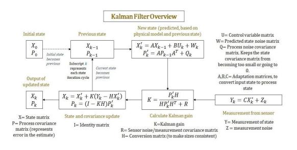
Figure 3.3. Kalman filter process flow chart [31]
