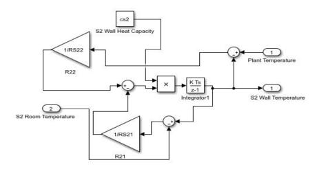
Figure 5.4. Exploded view of the S2 zone wall subsystem. The inputs to this bloack are the plant temperature and S2 room temperature and the output is the S2 zone wall temperature.R21 and R22 are the thermal resistances, cs2 is the thermal capacity of S2 zone wall
