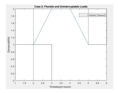
Figure 4.6. Optimal schedule was found for case 2 by operating the machines during the low demand periods
