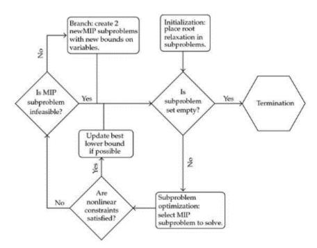
Figure 2.3. Branch and Bound algorithm flowchart
