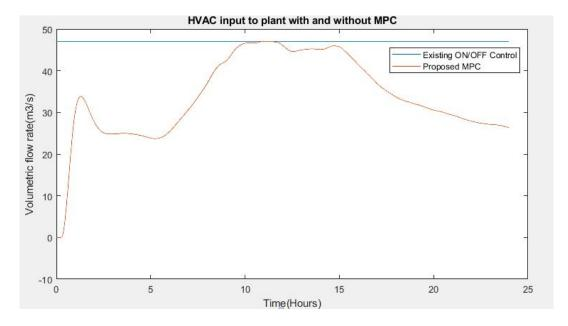
Figure 6.12. Controlled plant input flow rate using the MPC for a set point of  $296\mathrm{K}$
