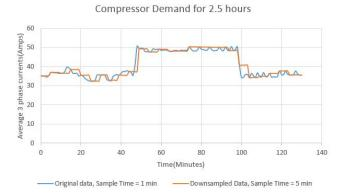
Figure 6.1. Compressor demand data sampled after down sampling
