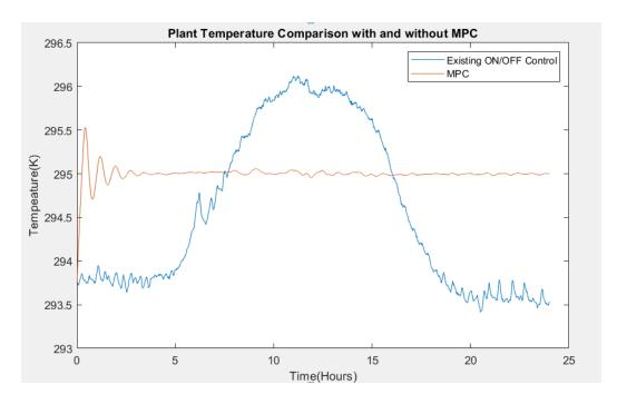
Figure 6.11. Controlled plant temperature using the MPC for a set point of 295K
