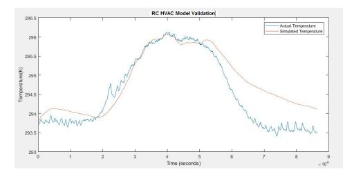
Figure 5.6. Comparison between the Actual Temperature of the plant and the model temperature for 1 day (86400 seconds) with the same input volumetric flow rate of  $47 \ m^3/s$
