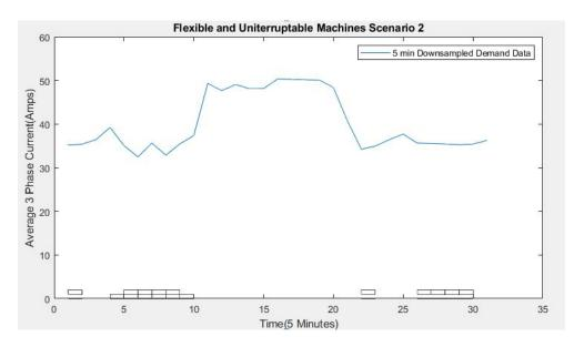
Figure 6.5. Optimal machine schedule for scenario 2 of Flexible and Uninterruptible machines case
