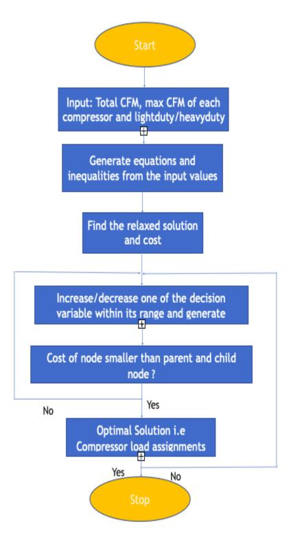
Figure 6.6. Flow chart for the Compressor Load Shifting problem
