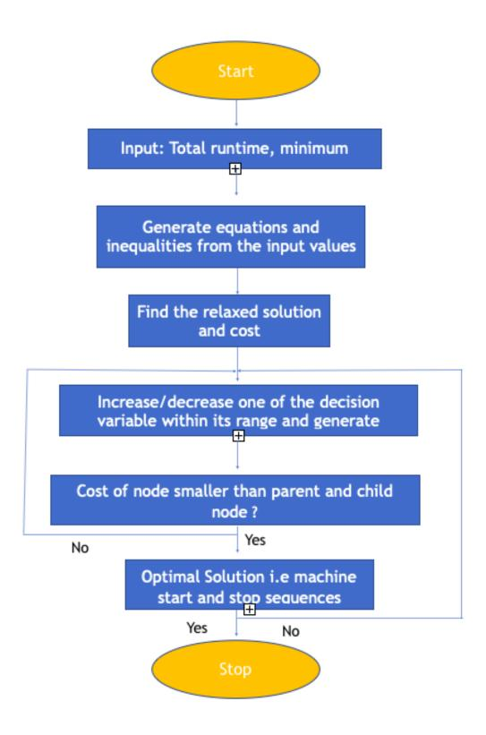
Figure 6.2. Flow chart of the Optimal Load Shifting problem
