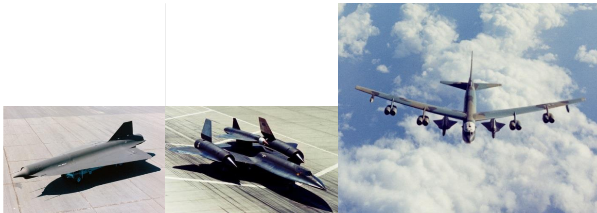
Fig. 11. The Tagboard drone alone, carried by an M-12, and two carried by a B-52. 122
