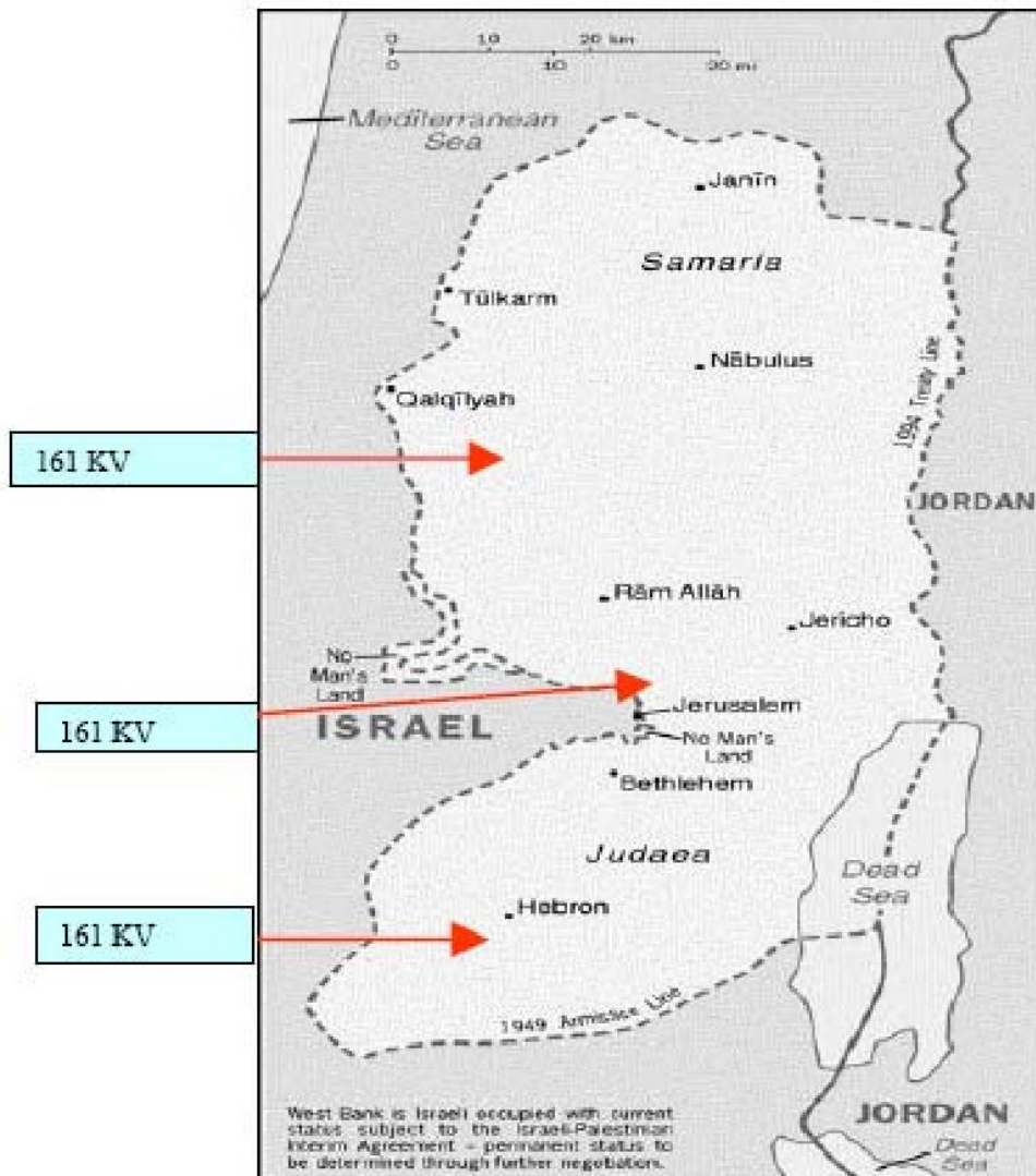
Figure 1.1: Main IEC Feeders to West Bank.
