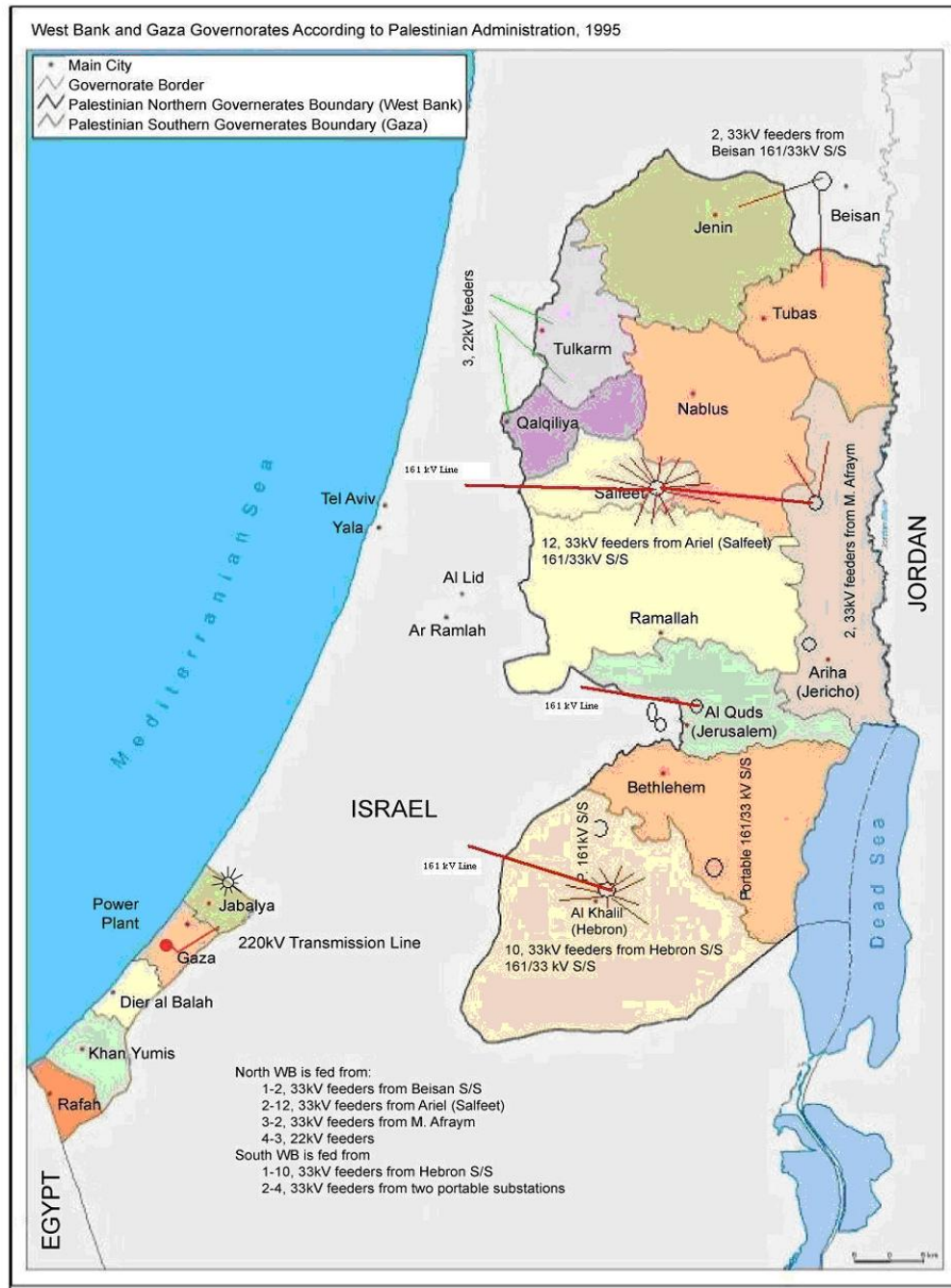
Figure 1.5: West Bank IEC MV cables supplying load centers.
