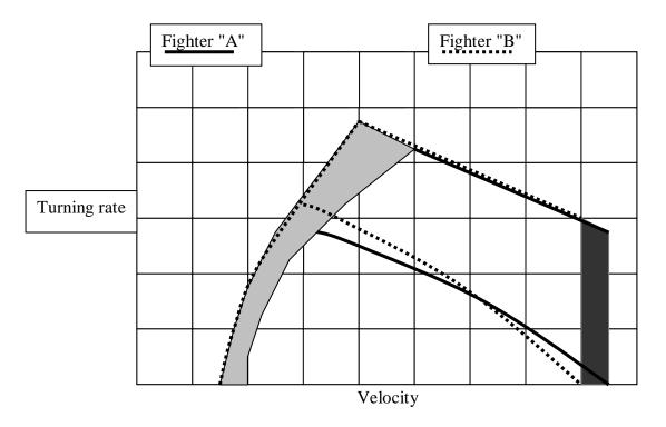
Figure 5.4. Horizontal Plane Performance Comparisons (The "Doghouse" Plot)
