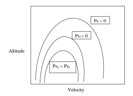
Figure 5.2. Specific Energy Rate for Typical Fighter Aircraft
