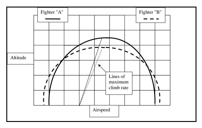
Figure 5.5. Vertical Plane Performance Envelope Comparisons for Airplane "A" and Airplane "B"
