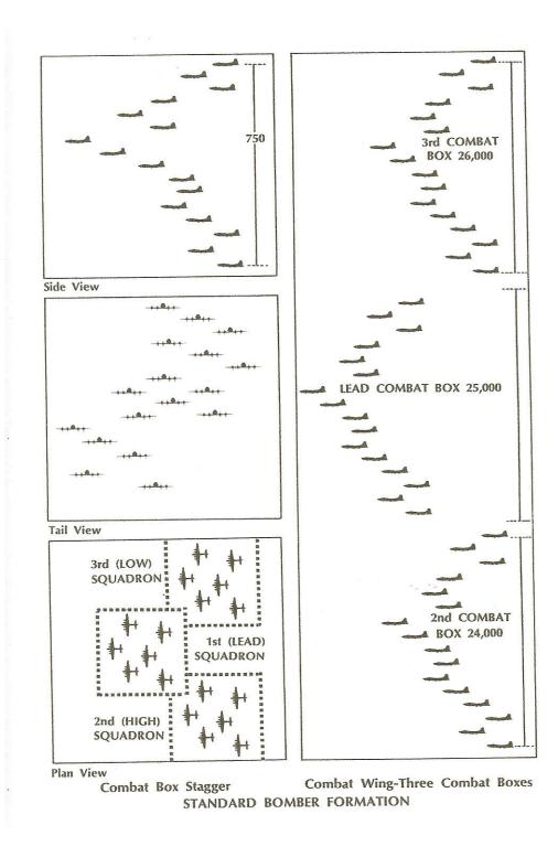
Figure 2.2 USAAF Bomber Formation Geometry (Ref. 14)
