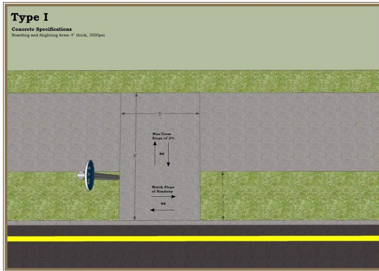
Figure 3-1. Type 1 Bus Stop Minimum ADA Compliance
