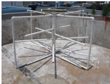
Figure 2.2: The in-tank component of the coral-sel, composed of the central column, mounting arms, support frame, guiding tubes, and attached bike wheel frame.
