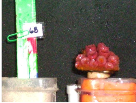
Figure 4.6: A Tubastraea coccinea colony utilized in the flume experiment. The colony is cemented to the ceramic pedestal.
