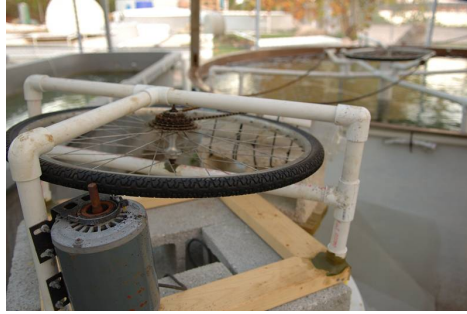
Figure 2.1: The motor and drive component of the coral-sel connected to the in-tank rotating component.
