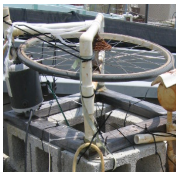
Figure 2.6: Close-up of the driving component of the coral-sel with its attached gears.
