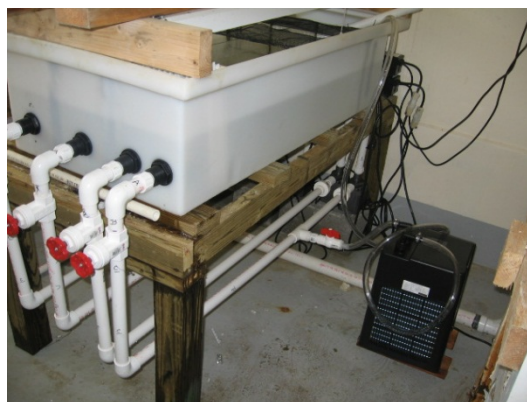
Figure 4.3: A semi-recirculating tank showing the connection of the electronic chiller to one of the high flow pipes. Note: Before the initiation of the experiment, the hose returning the chilled water to the tanks was repositioned to the “inflow” end of the tank to allow chilled water to be fed through the system before immediately being returned to the chiller.
