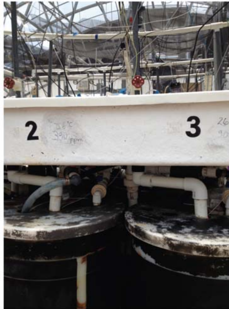
Figure 1.3. Schematic diagram (courtesy of R. Okazaki, C. Langdon and A. Baker) (a) and photographs (b,c) of CO 2 experimental system at the University of Miami Experimental Hatchery (UMEH) for culturing corals under controlled temperature and natural light. Elevated pCO 2 is achieved by mixing pure CO 2 with ambient air, then passing the gas through a Venturi injector into the 200 L sump tank. Water temperature is regulated with a sensor that turns on heating or countercurrent cooling as needed. Seawater from the sump tank circulates to the top holding tank and gravity feeds back into the sump
