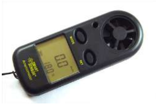
Figure (3.12): Smart sensor electronic anemometer.
