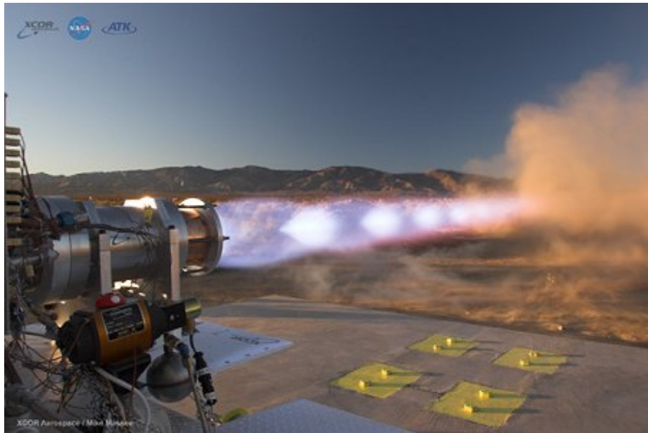
Figure 5.59. Test firing of a 7,500 pound-thrust LOX/methane engine. Image credit: Mike Masee/XCOR Aerospace. [106].
