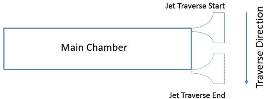
Figure 5.34. Schematic illustrating the position of the nozzle at the start of jet traverse and at the end [36].
