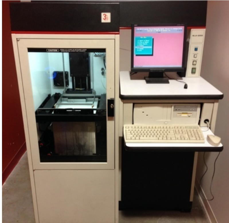
Figure 4.65 SLA Rapid Prototyping Machine Used To Create Module A and Module B Plastic Components
