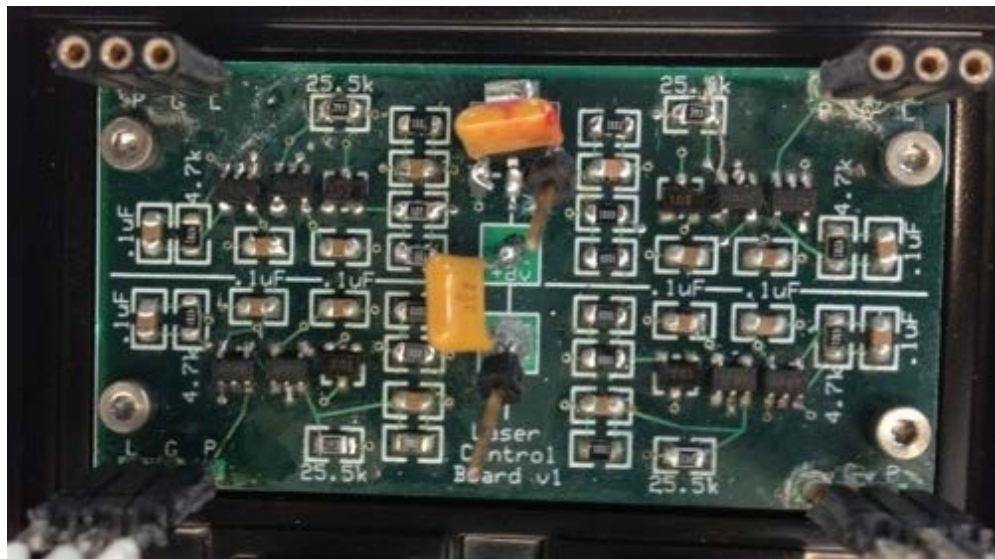
Figure 4.2(b) Module A Control Board Photo
