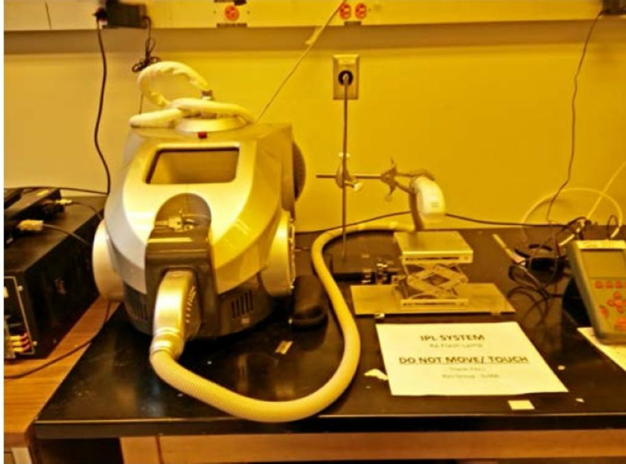
Figure 3.3. Image of commercial xenon flash lamp used in the study.
