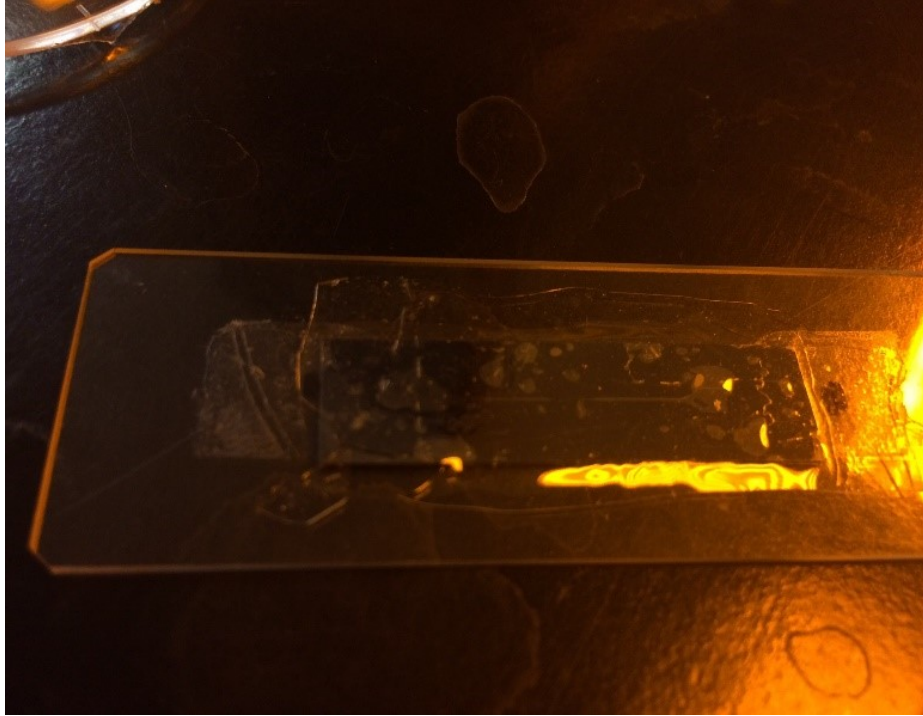
Figure 4.8. PDMS (Polydimethylsiloxane) sealed on the micro channels
