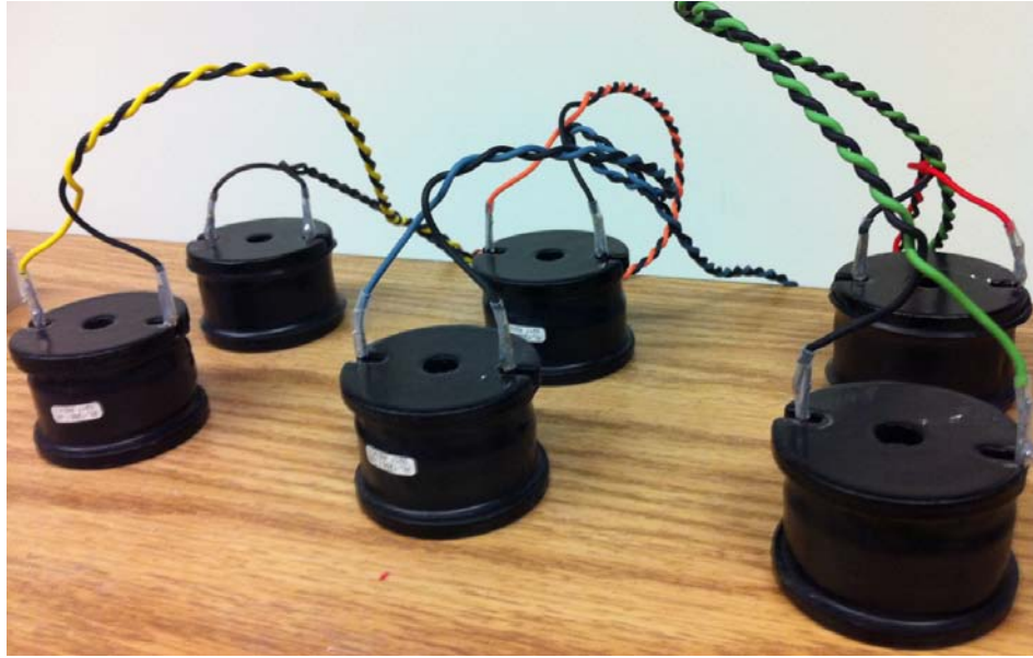
Figure 3.6 Inductors that emulates real injectors as load
