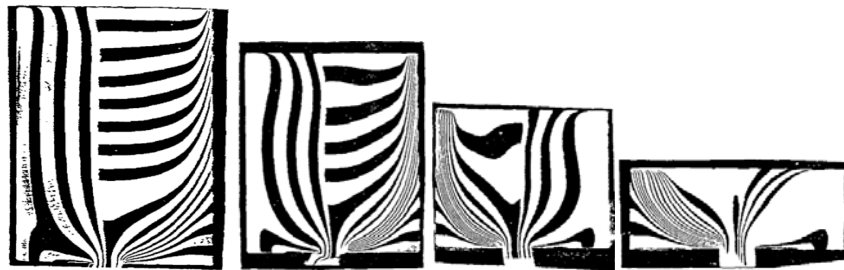
Figure 1.14 Transverse and longitudinal grid patterns used for the investigation of aluminum from during the whole extrusion cycle [13]
