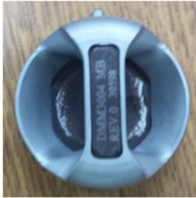
Figure 3.7 Image of modular die showing the wear pattern
