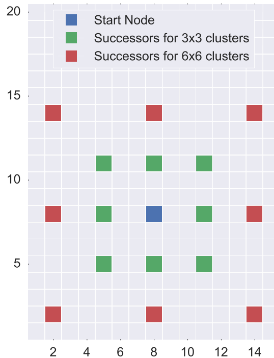
Figure 4.1: Improved method for determining hierarchical successors in 2D environments.
