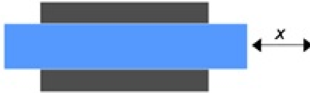
Fig. 2.14. Prismatic joint in 2D.
