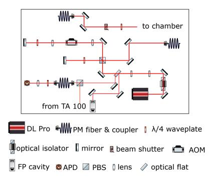
Figure 3.12. Optical layout for the imaging beam from DL Pro.
