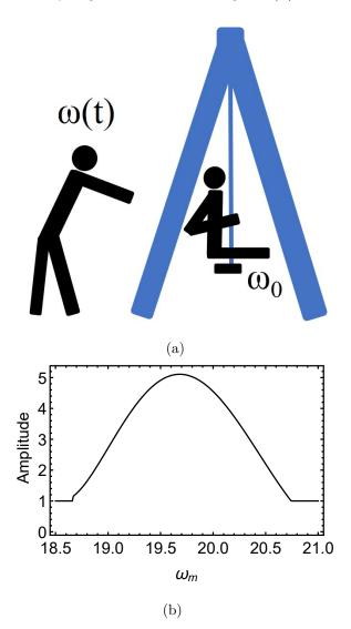
Figure 4.2. Parametric driving characteristics for a harmonic oscillator. (a) A child swinging at frequency  $\omega_0$ , being pushed at frequency  $\omega(t)$ . (b) Simulation of Eq. 4.1 with  $\delta = 0.15$ ,  $\omega_0 = 2\pi \times 10$  Hz, and  $t_m = 2\pi/\omega_m$ .
