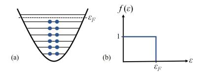
Figure 2.3. Degenerate Fermi gas energy characteristics. (a) Two-spin degenerate Fermi gas at zero temperature in a harmonic trap. (b) Fermi-Dirac distribution at zero temperature. At zero temperature the chemical potential equals the Fermi energy.
