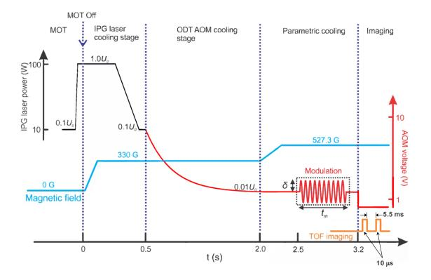
Figure 4.5. Experimental timing sequence. The sequence starts at the MOT loading stage where the ODT beam is first turned on, and ends after the two shots are taken for absorption imaging.
