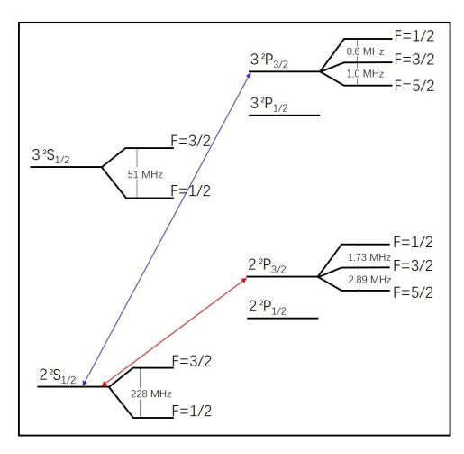
Figure 2.1. Partial hyperfine energy structure of <sup>6</sup>Li. The  $2^2S_{1/2} \leftrightarrow 3^2P_{3/2}$  transition (blue arrow) has wavelength 323.361168 nm, and the  $2^2S_{1/2} \leftrightarrow 2^2P_{3/2}$  (red arrow) is the  $D_2$  transition with 670.97738 nm wavelength.
