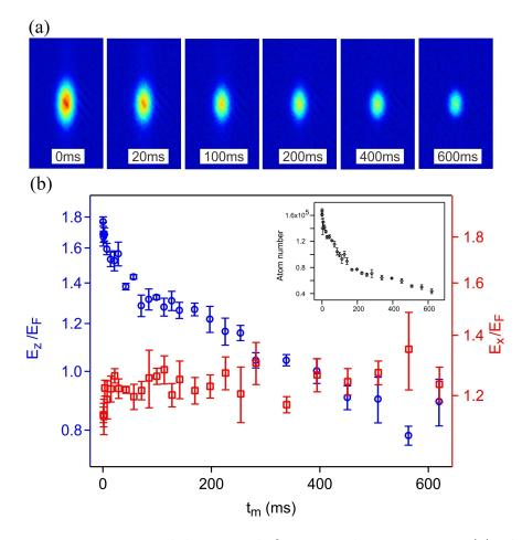
Figure 4.8. Time modulation with  $\delta = 0.5$  and  $\omega_m = 1.45\omega_x$ . (a) The absorption images of the atomic clouds of various modulation times. (b) The dependence of  $E(x, z)/E_F$  on modulation time (blue circles are for  $E_z/E_F$  and the red squares are for  $E_x/E_F$ ). The inset figure is the atom number versus modulation time. Error bars represent one standard deviation.
