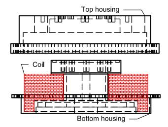
Figure 3.19. Schematic of coil and housing design. Water cooling of coils uses a water flow of about 3 gallons/minute.
