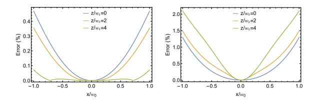
Figure 4.3. Deviation of the harmonic approximation from the actual trap in the x-direction as a function of position in the z-axis. (a) Harmonic approximation using the  $\omega_x(z)$  calculated from Eq.4.7. (b) Harmonic approximation using the  $\omega_x$  calculated from the trap depth as in Eq. 3.11.
