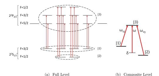
Figure 6.1. <sup>6</sup>Li –  $D_2$  Diagram. A  $\pi$ -polarized, monochromatic light stimulates both  $|1\rangle \rightarrow |3\rangle$  and  $|2\rangle \rightarrow |3\rangle$  transitions. The full level model in (a) is simplified to the composite level model in (b).  $\delta$  is the laser detuning from the transition between average of ground states to excited state. Energy levels are not drawn to scale.
