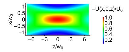
Figure 3.17. Trap potential of the crossed-beam ODT
