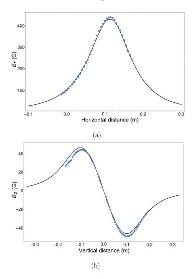
Figure 3.21. Measurement (blue points) and theoretical prediction (black lines) of one of the coils used for the MOT and Feshbach resonance magnetic fields. (a) Vertical measurement. (b) Horizontal measurement. The vertical magnetic field was measured using 120A current and distance was measured from the center of MOT (6.2 cm). The horizontal field was measured at a 7.6 cm vertical distance from the bottom with a 10 A current
