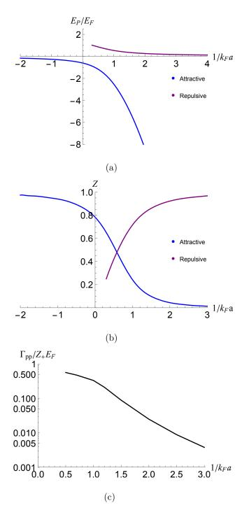
Figure 5.5. Three-dimensional polaron characteristics. (a) Energy spectrum. (b) Quasiparticle weight. (c) Lifetime of polaron against attractive polaron decay. The plots are based on theory from Refs. [108, 110].
