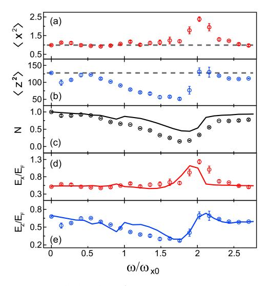
Figure 4.7. The dependence of parametric excitation on the modulation frequency. The radial and axial NIMS, the normalized atom number, and the radial and axial energies are shown from the top to the bottom. The harmonic frequency  $\omega_{x0} = 2\pi \times 740$  Hz is the measured value. The dashed lines indicate the average value without parametric modulation ( $\delta = 0$ ). The solid lines show the simulation results.
