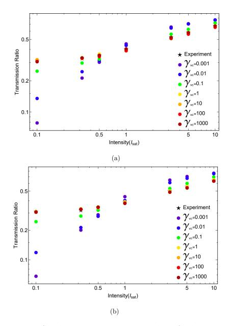
Figure 6.10. Simulation and experimental results at fixed beam power for (a) 60% transmitted power and (b) 80% transmitted power
