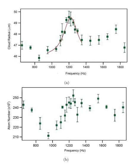
Figure 3.18. Trap frequency measurement in z-direction at  $0.1U_0$ . (a) is the cloud size obtained via a Gaussian distribution fit and (b) is the atom number.
