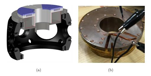
Figure 7.1. Magnet design and implementation. (a) Design for magnets to fit inside recessed window for closer proximity to trapped atoms with the red rectangles indicate the region of square wire windings. (b) Implementation of design on a water-cooled copper mount.
