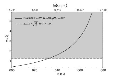
Figure 5.11. Ferromagnetic instability threshold in the gray region.
