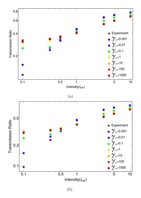
Figure 6.9. Simulation and experimental results at fixed beam power for (a) 20% transmitted power and (b) 40% transmitted power.
