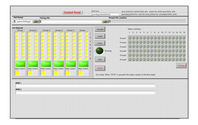
Figure 3.23. Main DAQ timing control for experiments. A timing file read by Labview sets the timing sequences.
