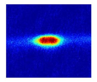
Figure 3.26. Absorption imaging of trapped atomic cloud in the horizontal direction. The cloud size is 42  $\mu$ m ×198  $\mu$ m with 2 $\theta$  = 14°.
