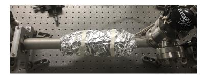
Figure 3.10. Vapor cell used for TA 100 frequency locking.
