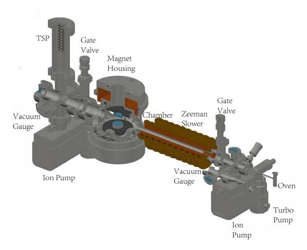
Figure 3.1. Vacuum system design. Not pictured is the non-evaporable getter material.
