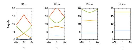
Figure 5.7. First Brillouin zone energy bands for a one-dimensional optical lattice created with laser of wave vector  $k = 2\pi/\lambda$ . The increasing trap depth creates smaller energy band depths with larger energy gaps.
