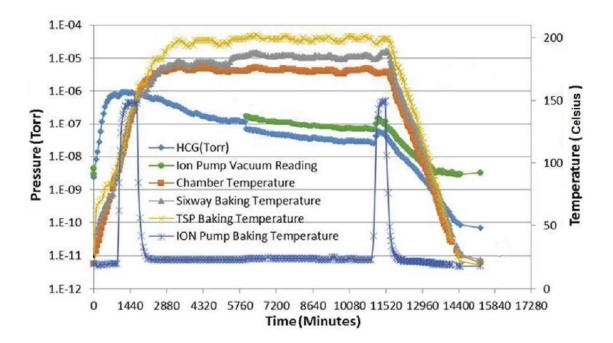
Figure 3.4. Pressure and temperature curves during bakeout.
