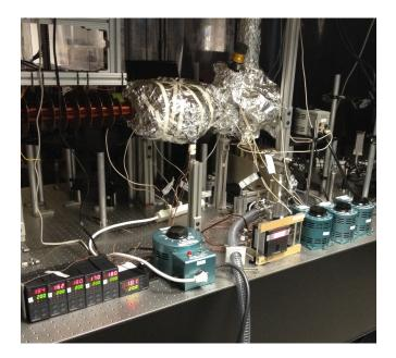
Figure 3.3. Vacuum system baking. Only the science chamber side is pictured; the same method of heating with heat tapes and aluminum foil was performed on the oven side.
