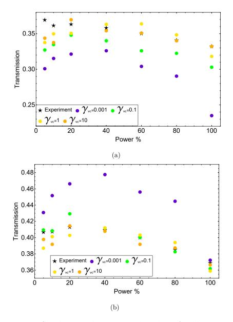
Figure 6.13. Simulation and experimental results at fixed beam power for (a)  $0.5I/I_{sat}$  transmitted power and (b)  $1I/I_{sat}$  transmitted power.
