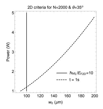
Figure 5.10. The region to the left of solid line does not satisfy the Fermi energy criterion; between the solid and dashed lines both conditions are satisfied; and region to the right of the dashed line does not satisfy the tunneling criterion.
