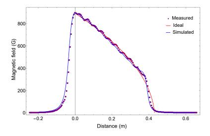
Figure 3.6. Zeeman slower magnetic field profile. A current of 9.6 A was used in all cases.
