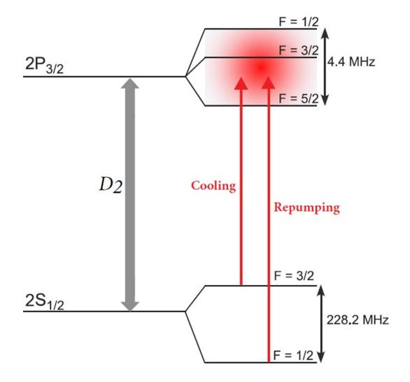
Figure 3.14. MOT transitions. The hyperfine splitting of the  $2^2 P_{3/2}$  states is smaller than the natural linewidth of the  $D_2$  transition.
