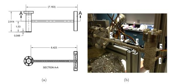
Figure 3.5. Lithium oven design and implementation. (a) <sup>6</sup>Li oven design with a rotatable flange on the oven nozzle and 1.33" flange on the top for lithium loading. (b) Oven mounted on apparatus with heating sections. Layers of high-temperature cement are used to separate the nichrome wires from the themocouples.
