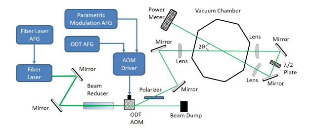
Figure 3.15. ODT control and optical layout.
