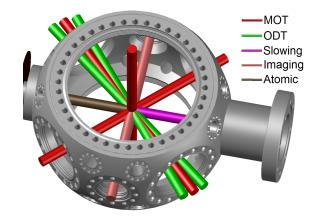
Figure 3.16. Optical and atomic beams in the science chamber. Beam sizes are not to scale.
