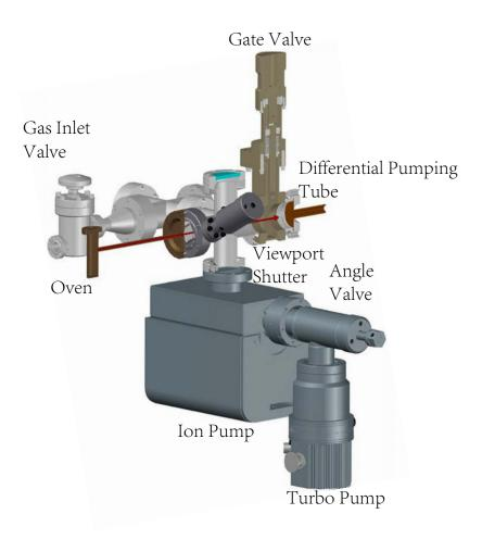
Figure 3.2. Oven side vacuum setup. The arrow indicates the atomic beam from the oven. An angle valve used during loading of <sup>6</sup>Li into the oven is shown to the left of the oven. An all-metal angle valve is used to connect a turbo pump into the system during initial pumping stages and baking. The differential pumping tube shown in copper color is used to keep the science chamber side at higher vacuum.
