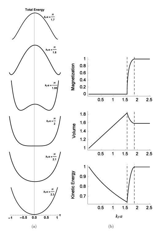
Figure 5.1. Stoner model properties for a three-dimensional system. (a) Total energy as a function of polarization. (b) Polarization, kinetic energy and volume. The kinetic energy is normalized to the total energy and the volume is normalized to the ideal gas volume. The dashed lines in (b) are for  $k_F a = \pi/2$  and  $k_F a = 3\pi/4\sqrt[3]{2}$ .
