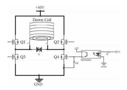
Figure 3.20. H-bridge circuit for the down coil. Each MOSFET has its own optoisolator and power supply. The optoisolators are used to protect the DAQ card from over current.
