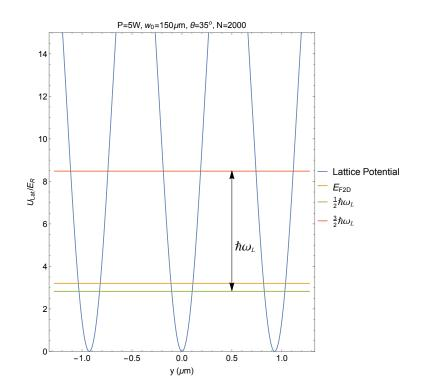
Figure 5.8. Lattice potential illustrating the relevant energies for confined two-dimensional motion.
