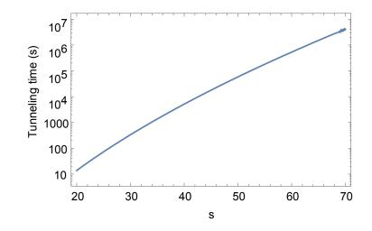
Figure 5.9. Tunneling time to adjacent pancake with  $2\theta = 35^{\circ}$ , and  $w_0 = 100 \ \mu m$ .
