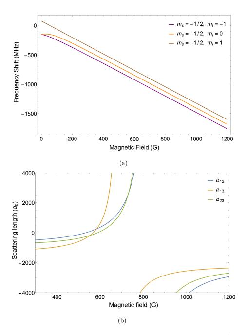
Figure 2.5. Energy states and Feshbach resonance profiles for <sup>6</sup>Li. (a) Energy shifts due to applied magnetic field for the three lowest energy states of <sup>6</sup>Li. (b) Scattering length dependence on magnetic field in terms of the Bohr radius for the lowest spin states. The narrow Feshbach resonance centered at 543 G for  $|1\rangle$ - $|2\rangle$  is not pictured.
