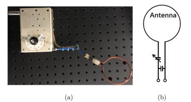
Figure 3.22. RF antenna. (a) Antenna with impedance matching circuit. (b) Circuit diagram for impedance matching circuit.
