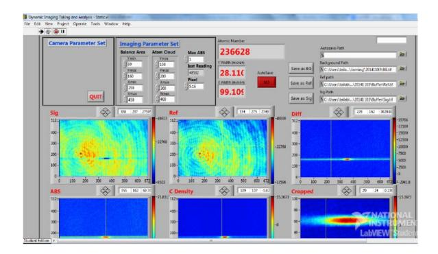
Figure 3.24. Sample image capturing and data analysis with LabView.
