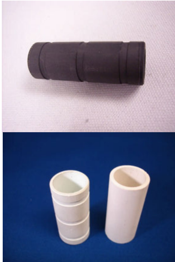
Figure 2-16 Porous pressure liners. New Way treated porous graphite (left), Aerodyn fabricated porous Alumina (right).
