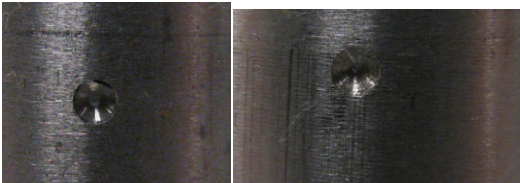
Figure. 2-18 Close up two feedholes 0.012" (left) and 0.006" (right).
