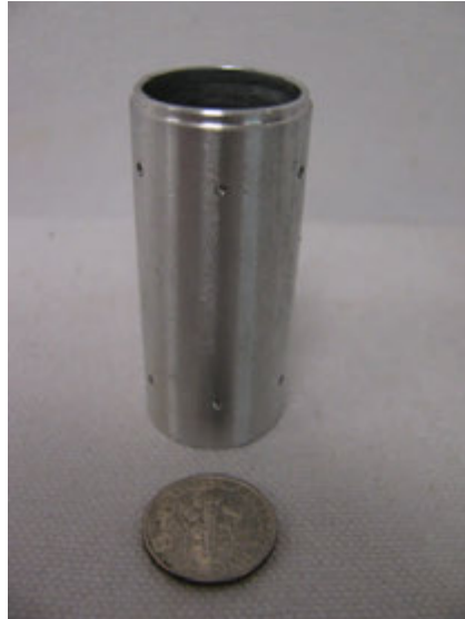
Figure 2-17 Feedhole mass addition pressure sleeve.
