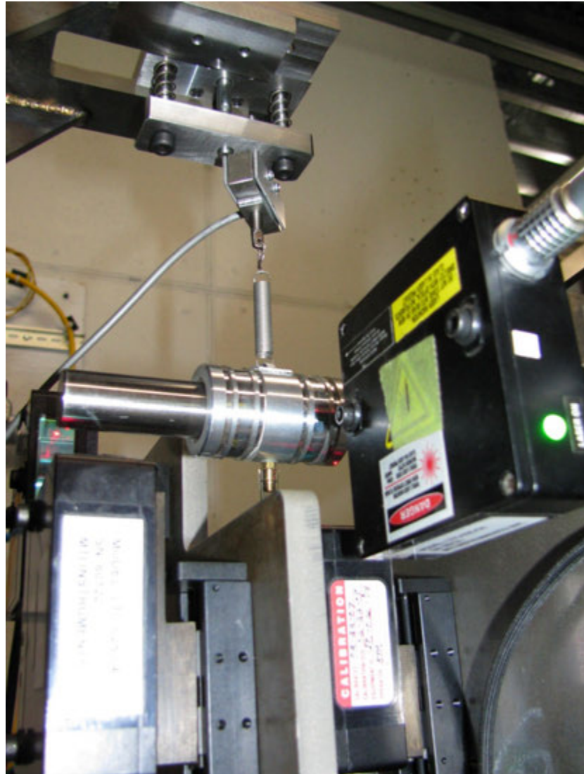
Figure 2-14 gas bearing test stand being used for static flight versus load testing.
