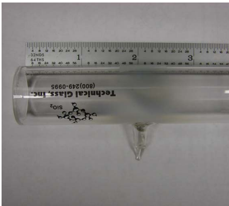
Figure 6.1. The paraffin cell used in our experiment.
