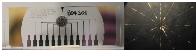
Figure 3.5: Electrode array with SWCNTs/PMMA (0.1% CNT) material (left) and an optical micrograph of the electrodes (right)
