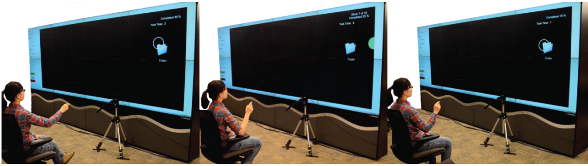
Figure A2. A user points in mid-air to a target folder on a large display (left); Stoppers provide visual feedback as the user's gesture goes out of the display range (center) and guide her back within the display range (right).
