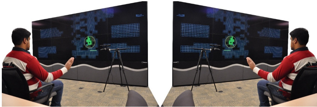
Figure 8.2. We studied handedness in touchless interactions with a circular steering-targeting task (same task used in the experiments evaluating interface topographies, Chapter 7). Right-handed users completed the task at a high level of density (high difficulty) on the large display while sitting at a distance.
