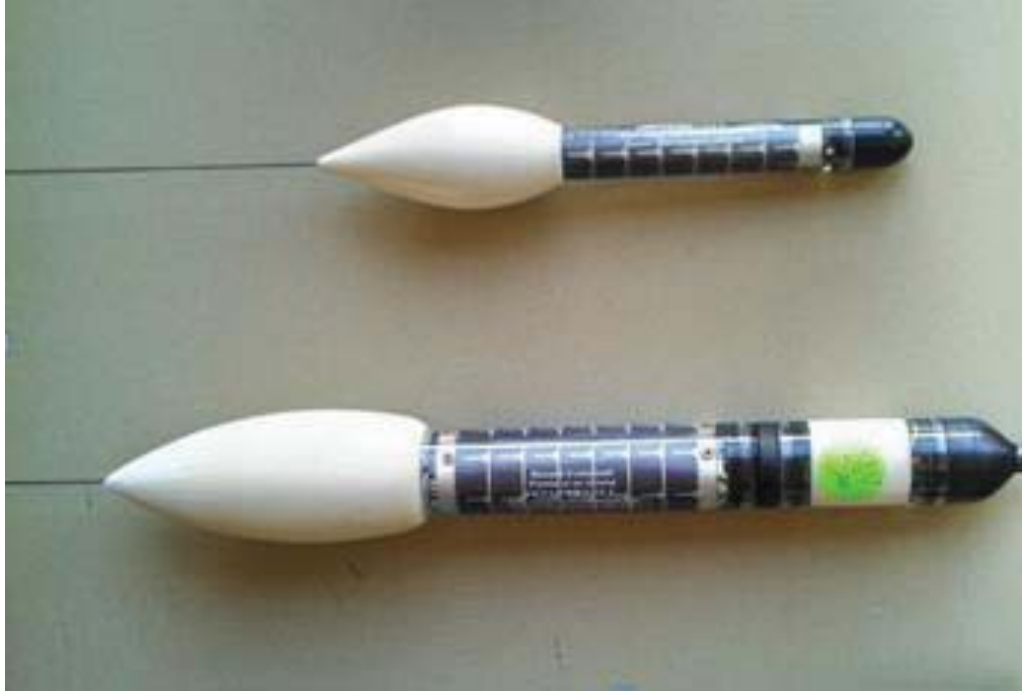
Figure 3.1: Top: SeaTag-GEO satellite tag used for long term deployments. Bottom: SeaTag-MOD satellite tag with attached battery section used for short term deployments and high-resolution data capture.
