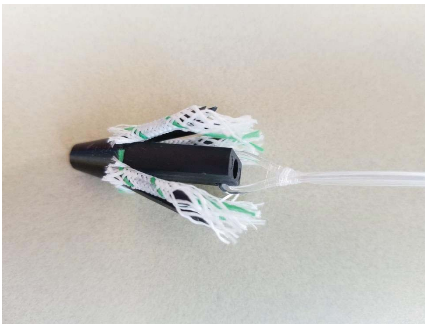
Figure 3.3: Enhanced view of Domeier dart with attached Dacron and applied heat shrink material over monofilament tether.
