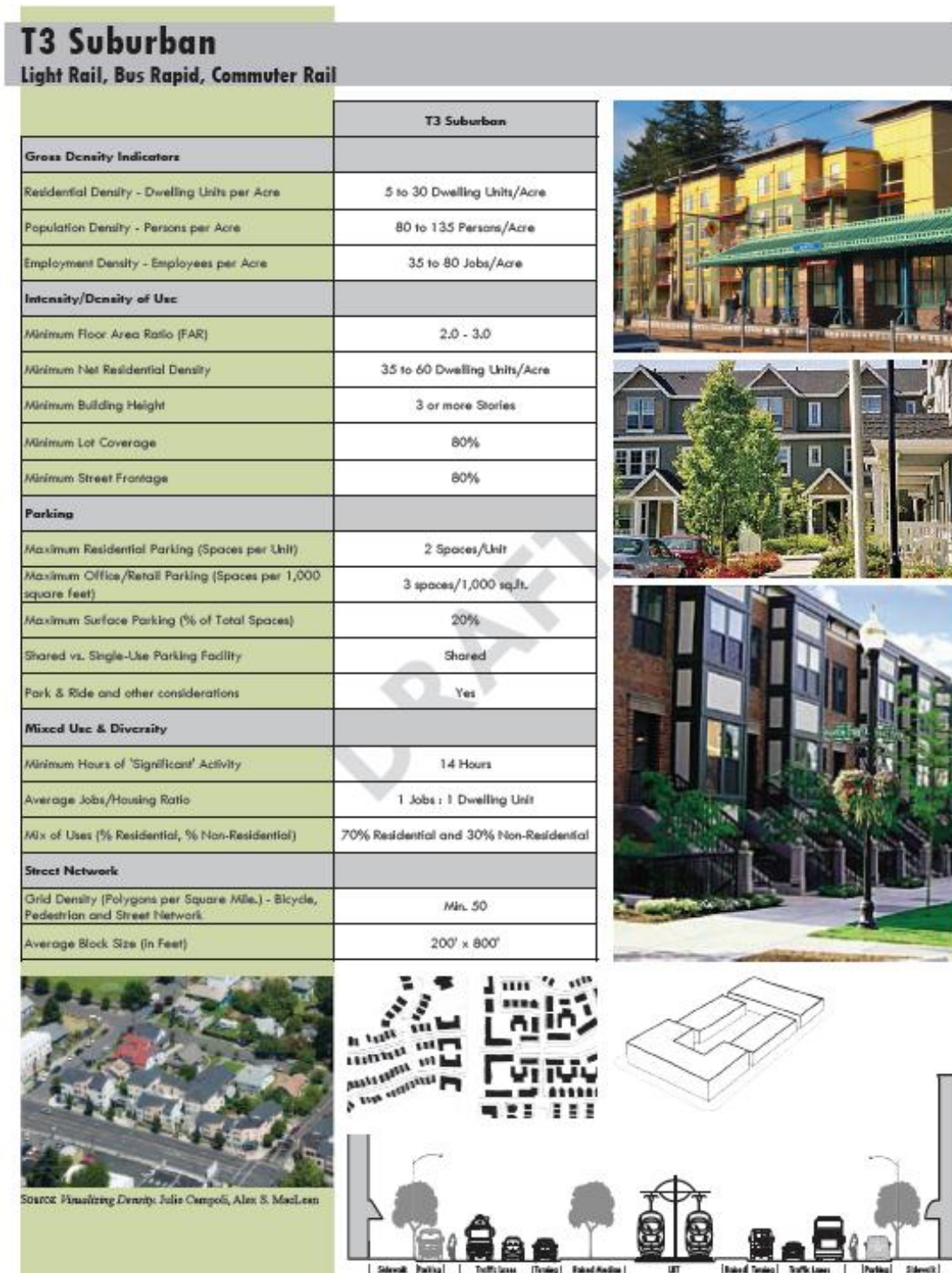
Figure F-1. Design standards by FDOT, Source - FDOT guidelines for TOD development
