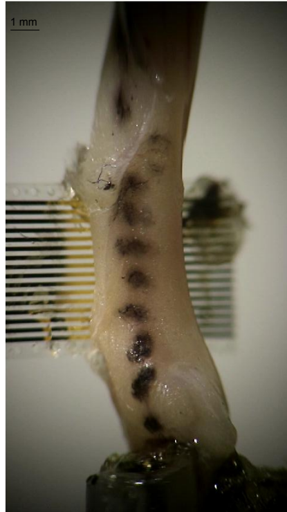
Fig. 4.4.: Image of the first frame of the tensile tests in the canine vagus nerve with an attached cuff and digital image correlation markers to show the location of the cuff.
