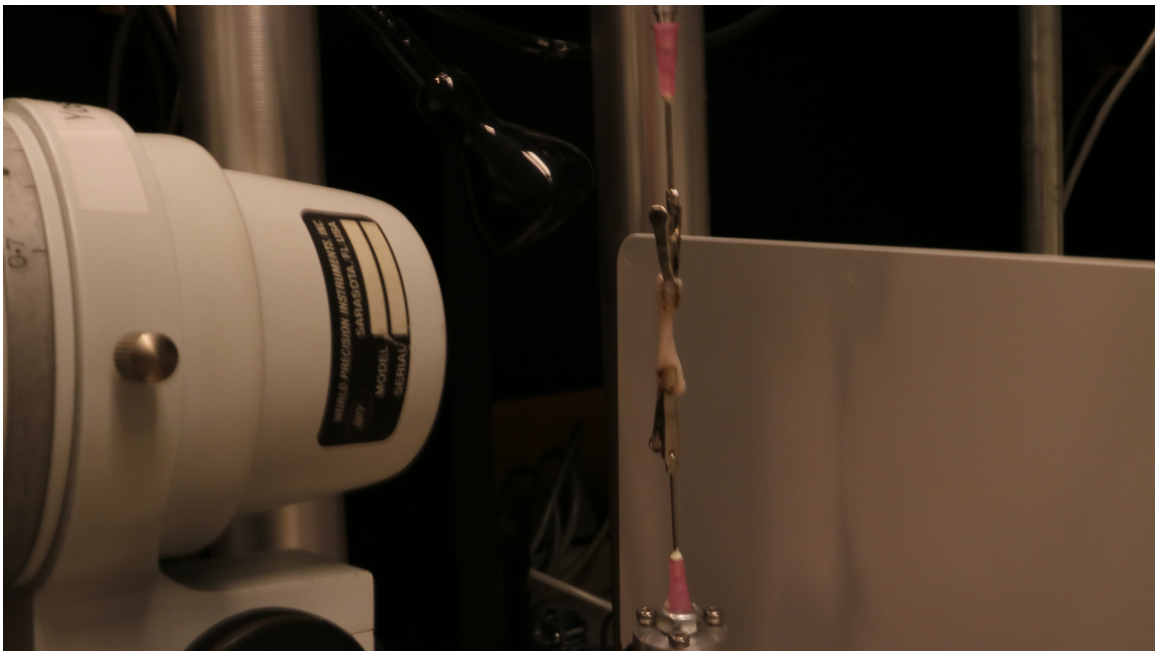
Fig. 3.5.: The fixture for tensile testing with a nerve fixed by alligator clips.
