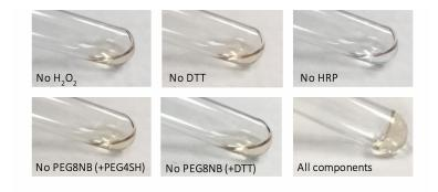
Fig. 4.1: Tilt test of HRP-mediated thiol-norbornene hydrogel. All components: 200 U/mL HRP, 0.5 mM  $\rm H_2O_2$ , 3.5 wt% PEG8NB, and 14 mM DTT.
