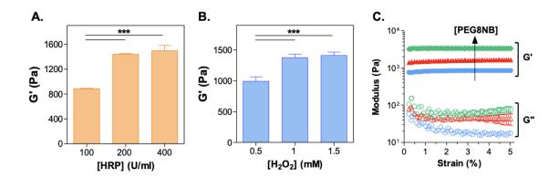
Fig. 4.4: Effect of (A) HRP concentrations and (B)  $H_2O_2$  concentration on shear moduli of PEG8NB-DTT hydrogels. Gelation was formed with 3.5 wt% PEG8NB, and 14 mM DTT,  $R_{thiol/ene}=1$ . N = 3, mean  $\pm$  SEM). (C) Strain-sweep rheometry of thiol-norbornene hydrogels formed with different macromer contents (3, 3.5, and 4 wt%.  $R_{thiol/ene}=1$ ). (n $\geq$ 3, Mean  $\pm$  SEM, \*\*\*p<0.001).
