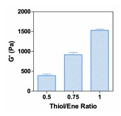
Fig. 4.16: 3 wt% GelNB-BA/3 wt% GelNB-HPA/PEG4SH hydrogels formed via LAP and UV-light (365 nm, 2 minutes) at different thiol-norbornene ratios.
