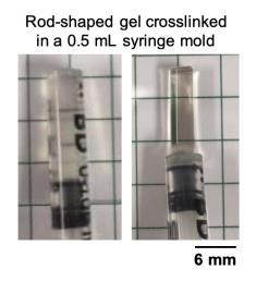
Fig. 4.5: HRP-crosslinked thiol-norbornene hydrogel with a diameter of 4 mm and and a length of 15 mm (200 U/mL HRP, 0.5 mM  $\rm H_2O_2$ , 3.5 wt% PEG8NB, and 14 mM DTT).
