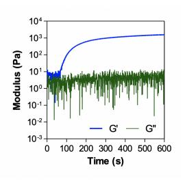
Fig. 4.2: In situ rheometry of HRP-initiated thiol-norbornene gelation (3.5 wt% PEG8NB, 14 mM DTT, 200 U/ml HRP, 0.5 mM  $H_2O_2$ ).
