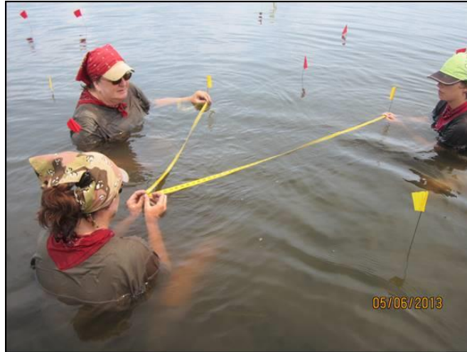
Figure 2.4. Photo of triangulating with a tape measure to set out an excavation unit on the sea floor. Photo by R. Watson.
