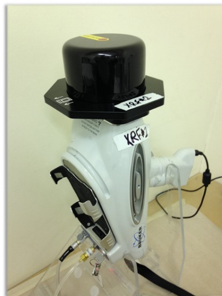
Figure 6. One of two Bruker AXS portable x-ray fluorescence machines used in sourcing of the obsidian.
