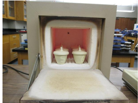
Figure 13. Photo of the inside of the furnace at 600 °C.
