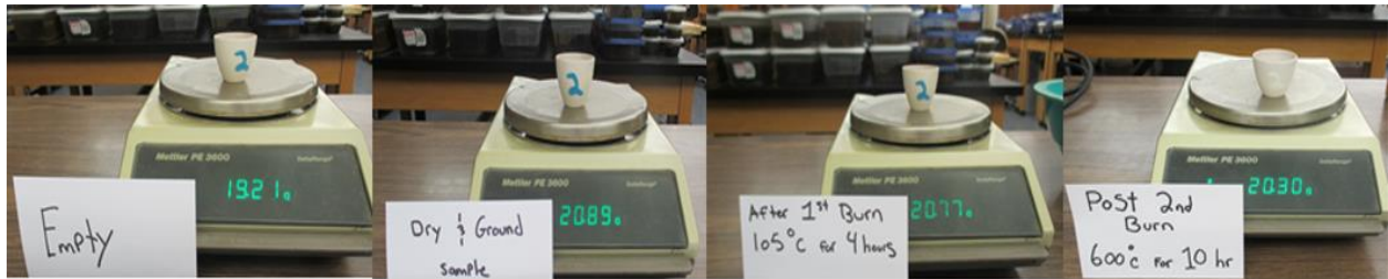
Figure 14. Photo showing the weight of sample 2 throughout the loss-on ignition process.
