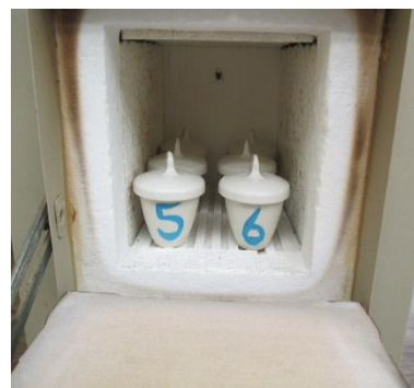
Figure 11. Photo of the inside of the furnace at 105 °C.
