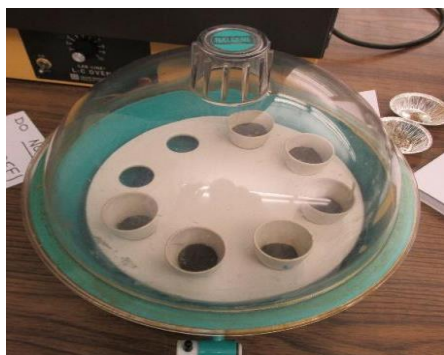
Figure 9. Photo of desiccator.
