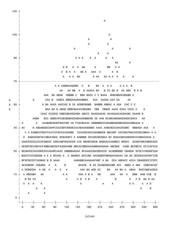
Figure 3.21 Daily O<sub>3</sub> maxima for Port Allen from the years 2000–2012 plotted against the Julian day with a reference line at the 75 ppb design value.
