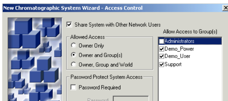
Figure 17, Instrument Access Control
