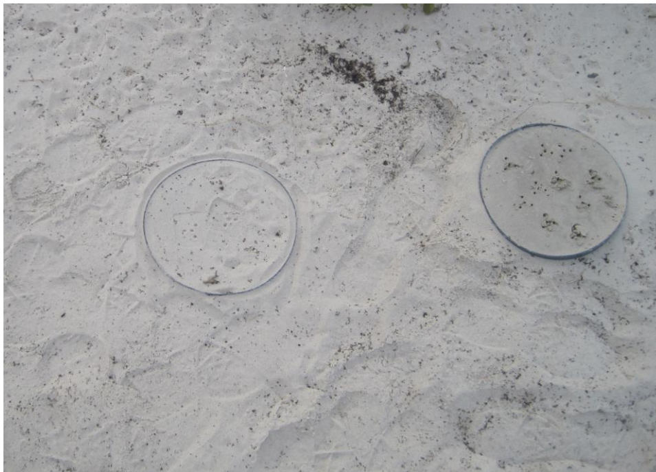
Figure 5.3: Picture of the evaporation trays taken in the field. Dry tray on the left, saturated tray on the right.
