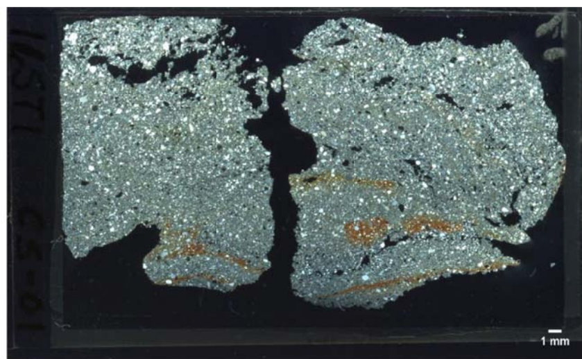
Figures 42 and 43 (L-R). Sample 17- Fired Clay Sample from near 16ST1. Left: Fired Clay Sample. Right: Cross-Polarized Scanned Image of Thin Section. Sample Collected by the Author.
